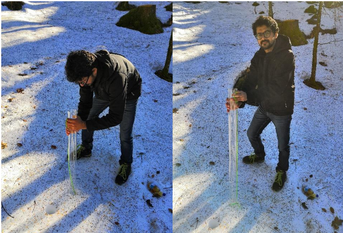
Figure A.3 Snow core sampling in the Dreisäulerbach catchment – (image credit: Michael Schäfer)
