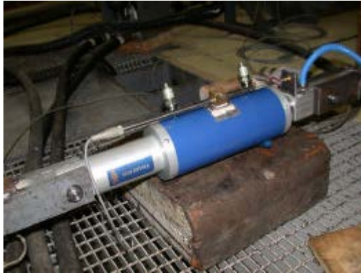
Figure 2-6. MR damper (Occhiuzzi et al. 2002)
