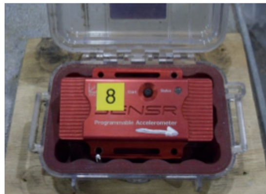
Figure 4-30. Accelerometer's installation (Pathan, 2021)
