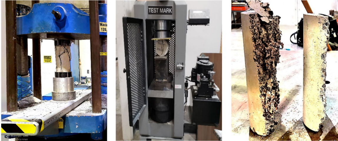
Figure 4-26. compression and tensile tests of TDA and concrete (Tehrani et al. 2020)
