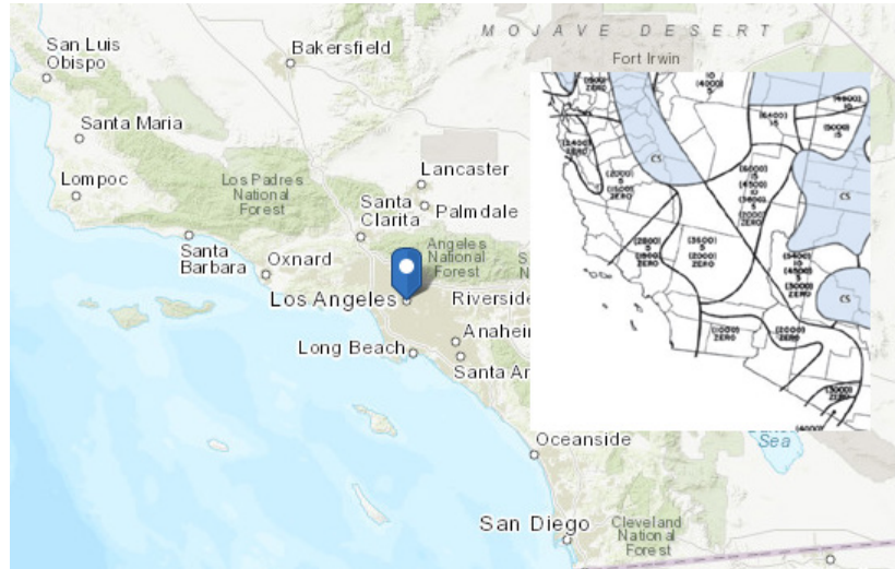
Figure 2. Ground snow loads, p_g , based on location ( \text{lb/ft}^2 , multiply by 0.0479 \text{ kN/m}^2 )
