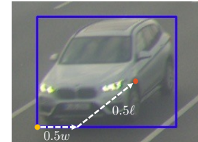
Fig. 3: Estimation of the object center (red) using predefined car extents w, \ell and the projected reference point (yellow).
