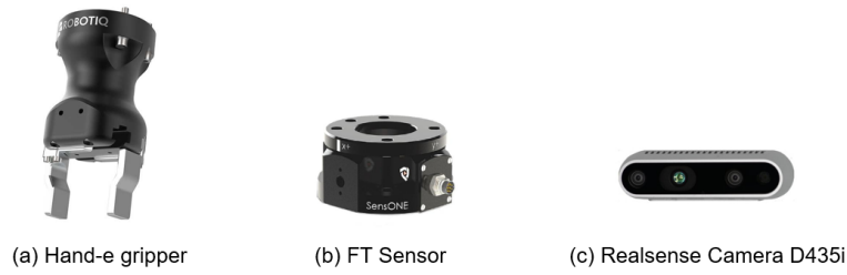
Figure 3.4: The new Hand-e gripper and the 6 axis force torque sensor and the Intel Real-sense camera.
