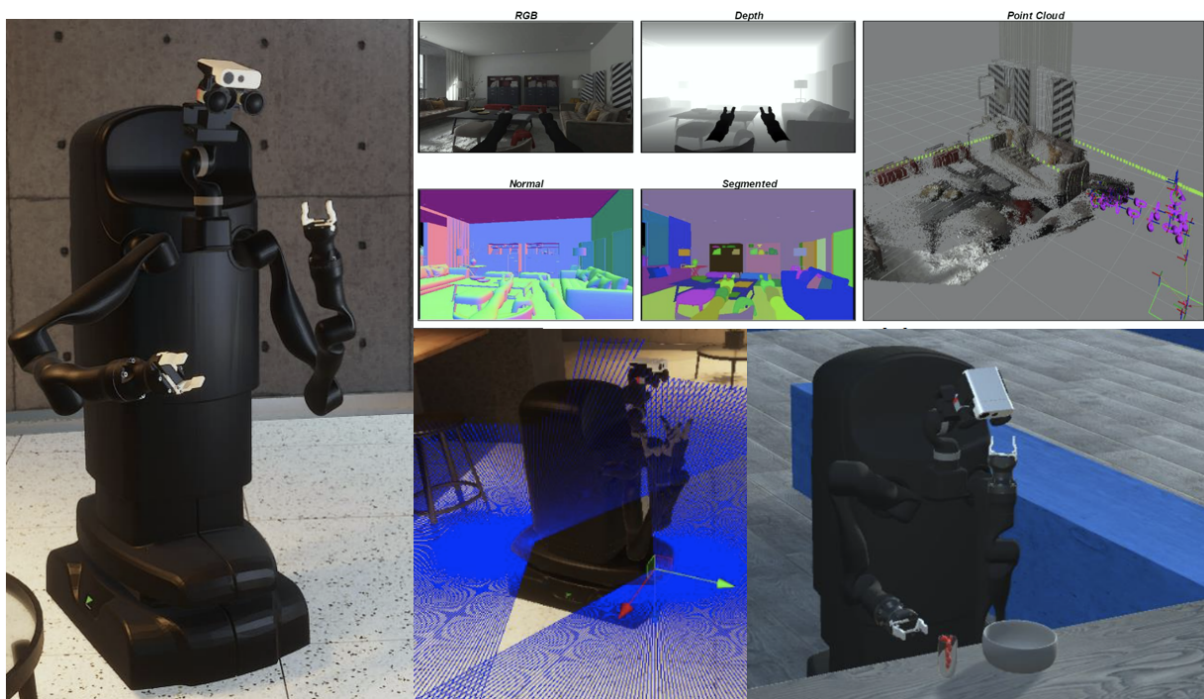
Figure 3.9: Photo realistic high definition rendering pipeline in Unity3D on the left and sensor outputs on the right. All the robot sensors such as IMU, LiDAR, cameras, depth cameras, transformations, and joint force and position feedback are provided to the ROS side through RRS.
