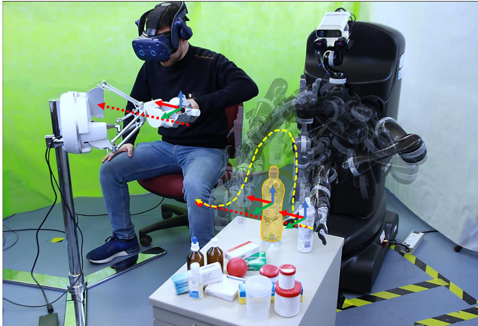
Figure 4.1: Real-time motion planning for dual-arm Kinova ® Movo platform using the proposed NMPC-MP for low-level shared autonomy in teleoperation. The orange object is the obstacle, and the dashed-red arrow denotes the desired motion. The dashed-yellow trajectory is the generated motion in order to avoid the obstacle. [1], ©2021 IEEE.
