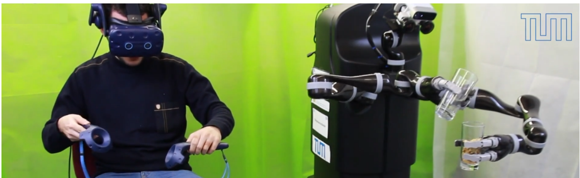
Figure 1.1: Dual hand liquid pouring. One of the basic requirements of a dual arm motion planning system is self-awareness. In a sense, each manipulator is a dynamic obstacle to the other. [1]
