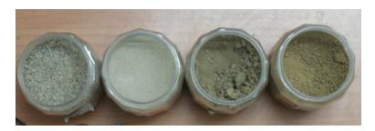
Figure 3.2: The four different soils used the study. From left to right: Soil 1: Grade I Sand (Bureau of Indian Standards (BIS), 2002), Soil 2: Grade III Sand (Bureau of Indian Standards (BIS), 2002), Soil 3: Silty-loam soil from local field, Soil 4: Graded Silty-loam soil.
