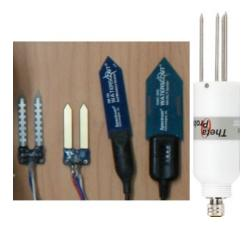
Figure 3.1: The four soil moisture sensors investigated in the study; from left to right (in the order of ascending cost): YL69, YL100, SM100, and SMEC300. The rightmost sensor is the secondary standard sensor, ThetaProbe.
