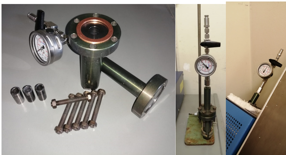
Figure 2.3. Picture of the disassembled autoclave (left) for reactions under hydrogen pressure. The assembled autoclave with the crucibles and reactants inside is depicted in the middle, ready to be loaded with hydrogen pressure. The hydrogen-loaded autoclave, placed in a tube furnace with stone wool for isolation is depicted on the right. A burst protection is adjusted in front.
