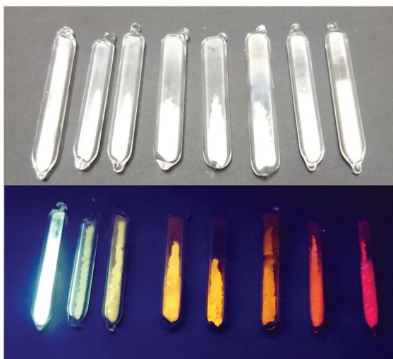
Figure 1. Photographic images of the solid solution series \text{CsCaH}_x\text{F}_{3-x}:\text{Eu}^{2+} ( x \leq 2.5 ) under day light (top) and the corresponding emission glow under 376 nm UV irradiation (bottom). (From left to right: x = 0, 0.25, 0.5, 0.75, 1.0, 1.5, 2.0, and 2.5 .)
