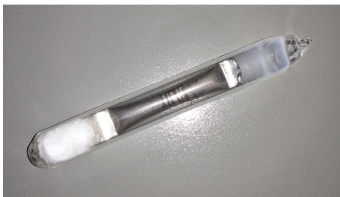
Figure 2.1. Picture of an encapsulated and sealed Ni-alloy ampoule, ready to be placed in an oven. Stone wool is placed as buffer between the quartz glass and the ampoule.
