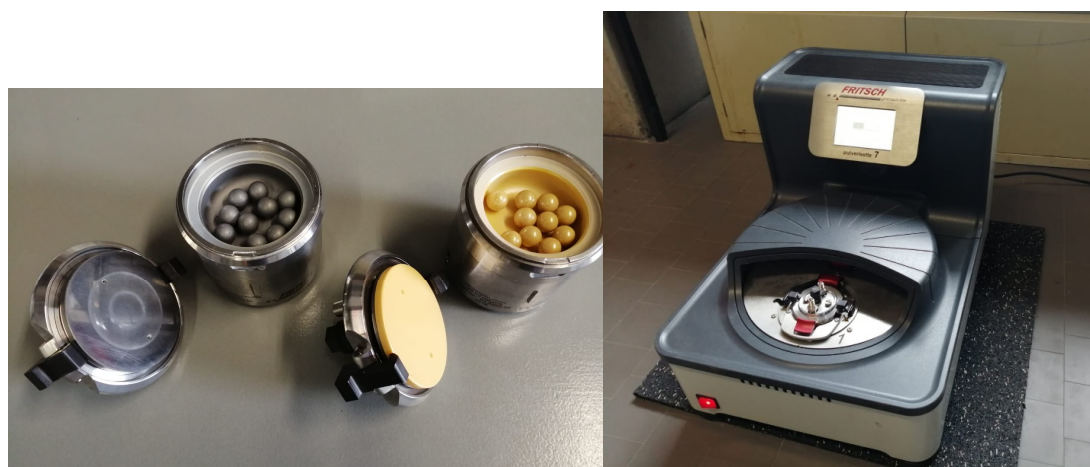
Figure 2.4. Tungsten carbide (grey) and zirconium dioxide (yellow) beakers with 10 balls each for mechanochemical reactions. Placed beaker in the planetary mill, ready to be started.
