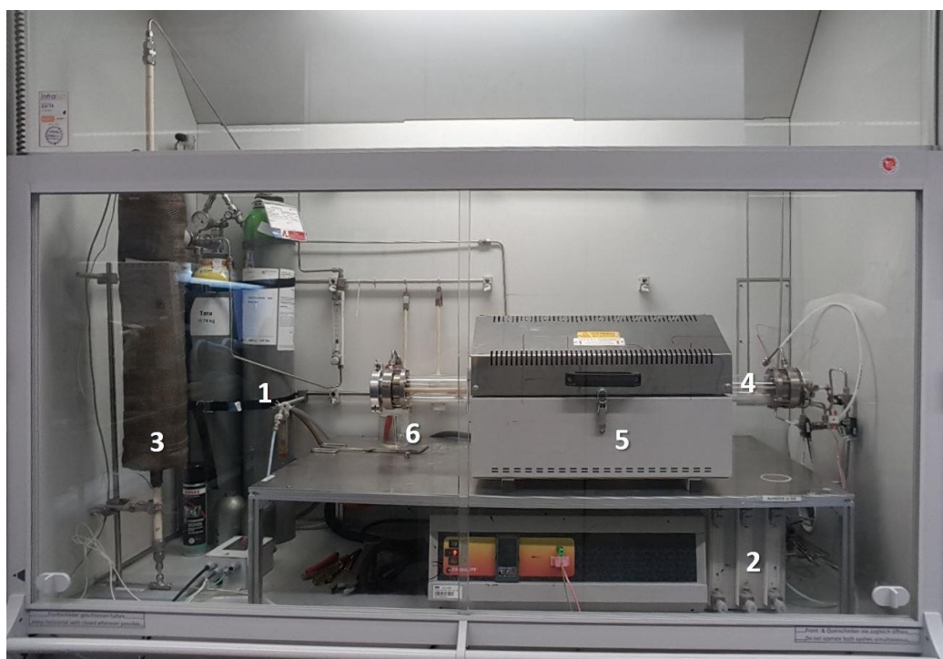
Figure 10: Photograph of the tube furnace setup for the SO 2 and SO 3 treatment of LMR-NCM samples. A detailed description and scheme can be found in Figure 3 in the experimental part of the publication 134 presented in chapter 3.3.1. A mixture of 1% SO 2 in Ar was provided by a 10 L gas cylinder (1). Ar, O 2 , and SO 2 in Ar were mixed via flowmeters (2) to reach a resulting flow of 1.0 l/min in the ceramic tube filled with the V 2 O 5 catalyst (3). The resulting SO 3 -containing gas mix then entered the glass tube (4) of the split tube furnace (5). The exhaust gases were then quenched by water in a washing bottle (6).
