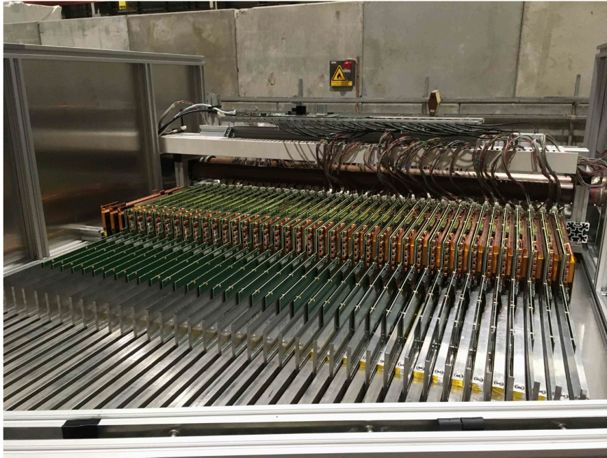
Figure 4.1: Fully assembled AHCAL technological prototype. The active layers, identified by the visible interfaces, are placed between the stainless steel absorber structure. In total the prototype consists of 39 layers.
