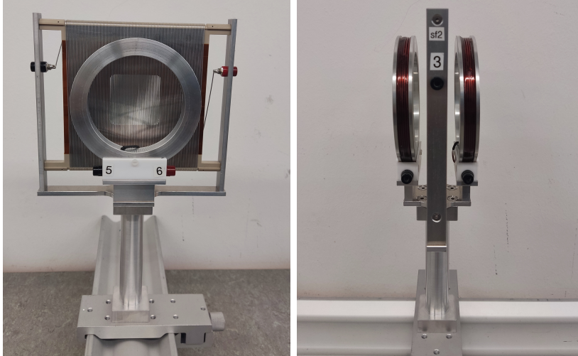
Figure 3.10: A \pi/2 -flipper consists of two perpendicular magnetic fields. The vertical field is generated by a rectangular Al coil. The horizontal field is generated by a Helmholtz configuration.
