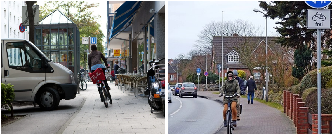
(c) Textural separation, cyclists could swerve onto the sidewalk (Peljak, 2018) and pedestrians (Hertel, 2019)
