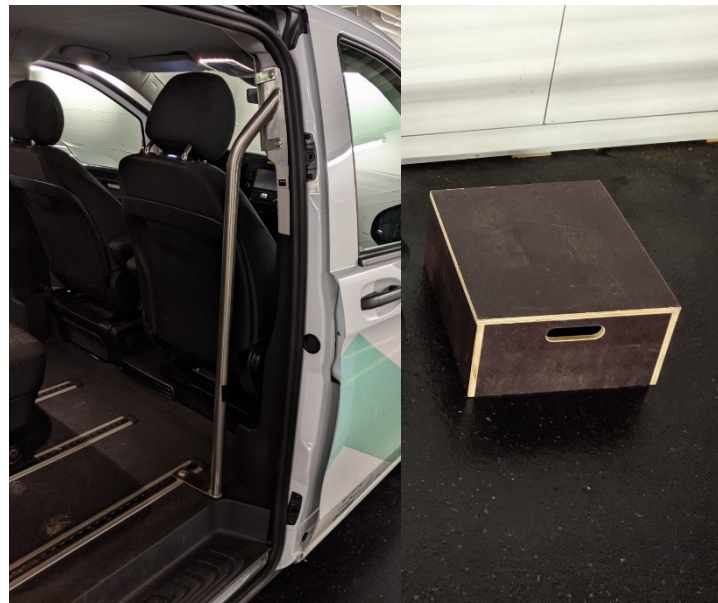
Figure 3. Necessary conversions because conventional series-production vehicles do not fully meet the required specifications (image rights are held by Pikmi (VBZ)). The provider in Zurich carried out the conversion work in 2021 after it had consulted on the suitability for everyday use in an internal workshop.
