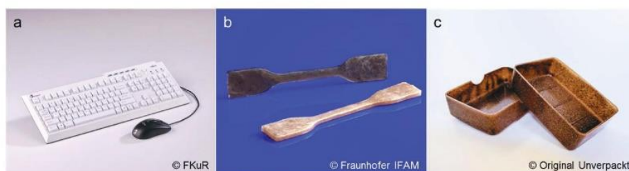
Figure 2. Examples of processed thermoplastic biopolymers from cellulose, chitosan, and lignin. From left to right: a) Computer keyboard and mouse injection molded from cellulose acetate. Reproduced with permission. [34] Copyright 2018, FKUR Kunststoff GmbH; b) injection molded tension rods made of chitosan. Reproduced with permission. [35] Copyright 2010, Fraunhofer IFAM; and c) injection molded soap dish using lignin-based ARBOFORM. Reproduced with permission. [36] Copyright 2019, Original Unverpackt GmbH.
