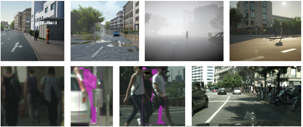
Figure 1: Examples of different factors contributing to the possible performance drop of the DNNs. The top row examples are from the KI-Absicherung dataset which include distance, wetness, fog and contrast factors. The bottom row examples are from the CityPersons dataset, which include brightness, occlusion, crowdedness and distance factors.
