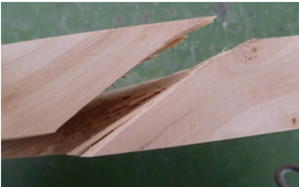
Figure 4: Maple specimen, failure at the slope of grain.
