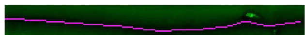
Fig. 4 Minimum of the RT profile representing the fibre for the European ash ( Fraxinus excelsior L.) specimen 263
