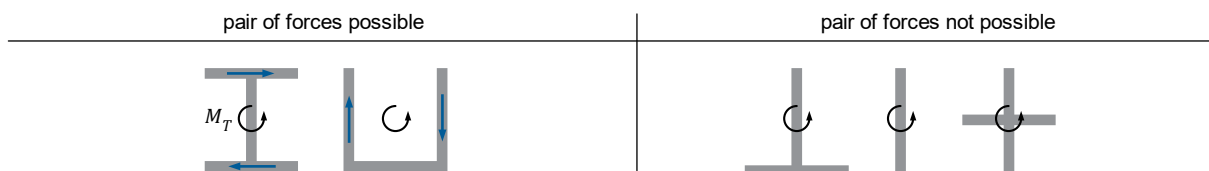
Figure 14 Thin-walled profile shapes that can activate a pair of forces (left) or not (right)
