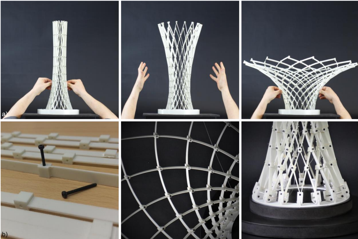
Figure 125 Model 1:10 of the Kinetic Umbrella with centric hinge axis.
