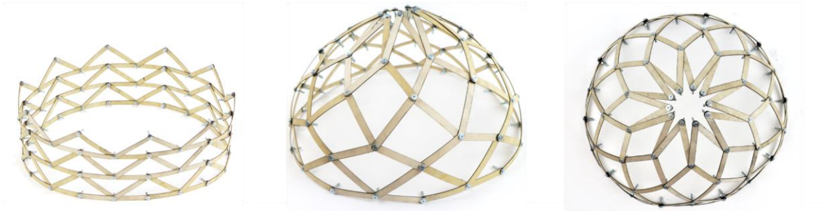
Figure 88 Physical Exploration of rotational symmetric scissor grids using angulated units on a cylindrical reference surface.
