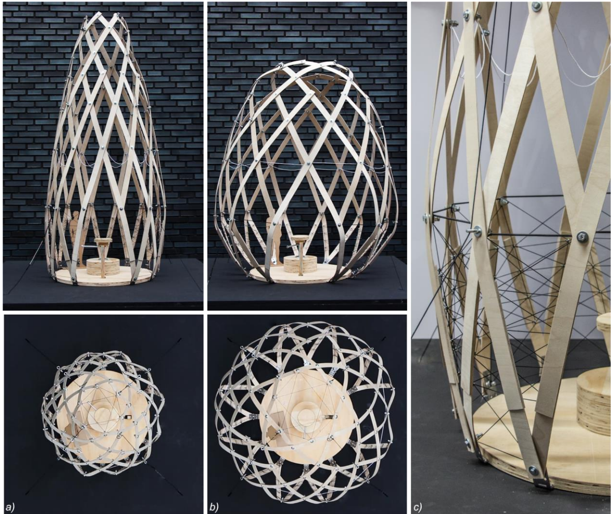
Figure 79 The Blooming Flower , a geodesic rotational grid structure: a) Open (bulgy) state – side and top view, b) Closed (slender) state, c) Details at support, locking cable (white) and supporting elastic actuation cables (black) (Photo: C. Saccomanno, N. Thierens)
