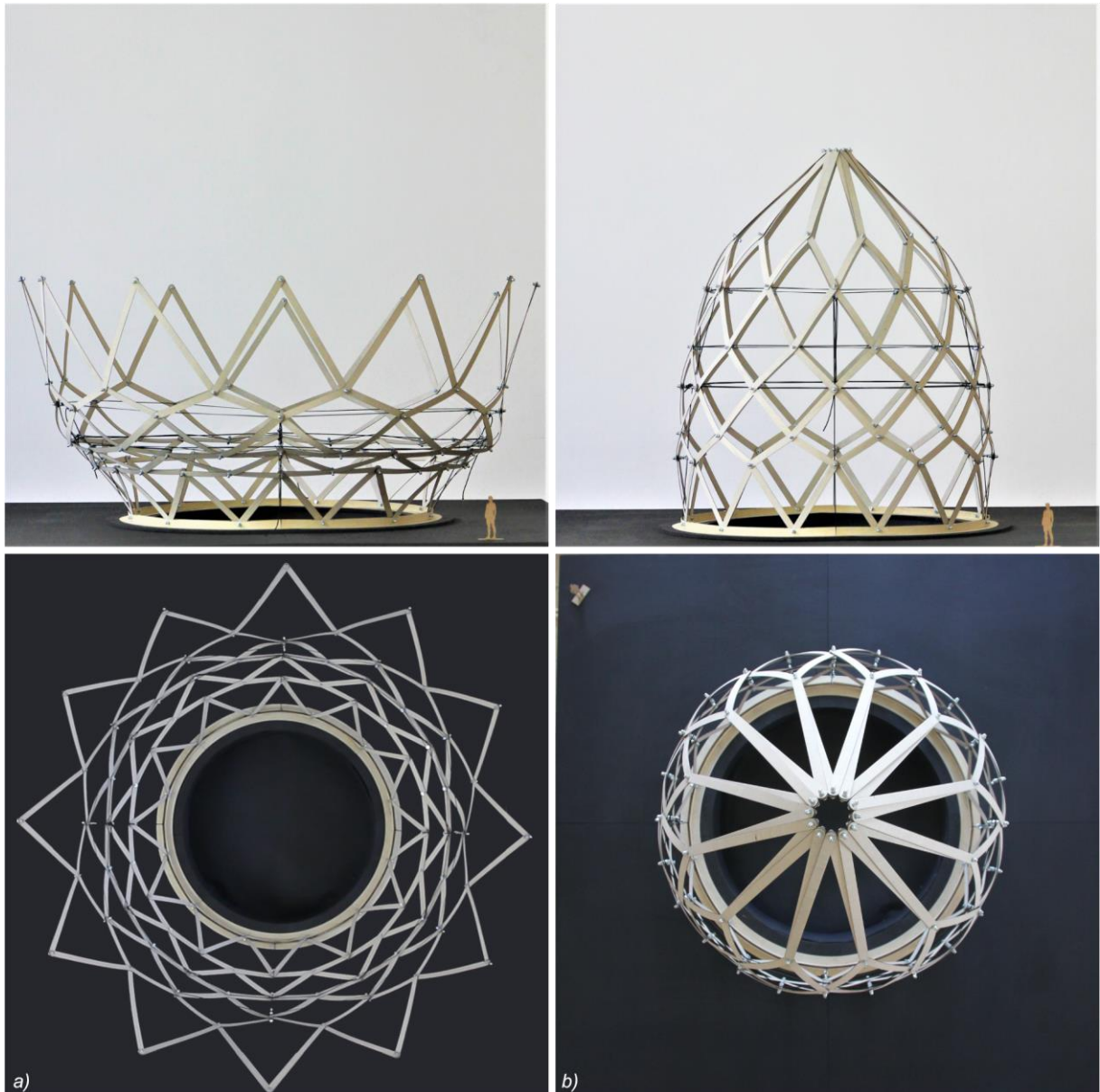
Figure 87 The EXX-dome, designed by Alberto Ortensi. The structure is actuated by highly elastic, (horizontally) and retractable cables (meridian): a) Open state, b) Closed state.
