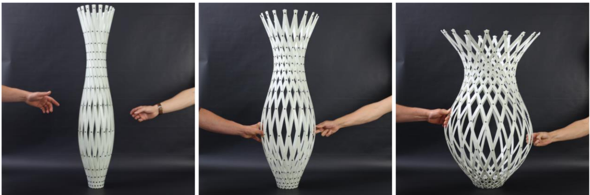
Figure 81 Physical model and three states of deformation of a rotational geodesic grid structure. The surface of this demonstration includes both synclastic and anticlastic surface areas.
