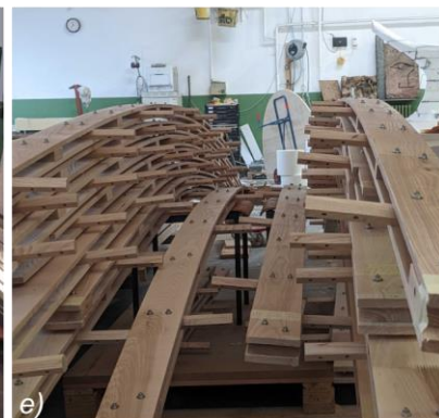
Figure 114 The Asymptotic Geodesic Timber Vault: a) View of the structure without cladding, b) Top view, (asymptotic curve set), c) Detailed view of the grid (web), including asymptotic (“upright”) lamellas and geodesics (“flat”) lamellas d) Shaping the grid structure from flat to spatial. e) Prefabricated curved, doubled lamellas.
