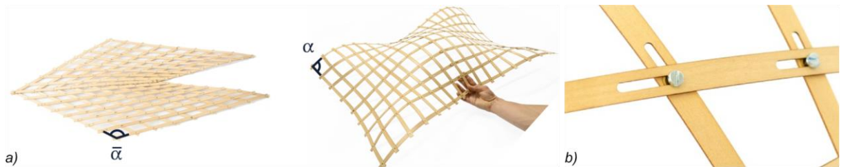
Figure 50 Physical model showing a) Flat to spatial deployment of a geodesic grid, b) Notches, necessary to provide a translational DoF at nodes to allow transformation (Pillwein, Kübert, et al., 2020)
