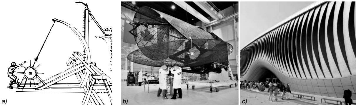
Figure 39 Various applications of compliant mechanisms: a) Compliant catapult, sketched by Leonardo da Vinci (Howell, 2001, p. 9), b) Inextensional deformation of the “Spring-Back Reflector” used for the M-SAT2 satellite (Tan & Pellegrino, 2006) c) Thematic Pavilion at the Expo 2012 in South Korea by SOMA architects and Knippers Helbig (Schleicher, 2016, p. 48)
