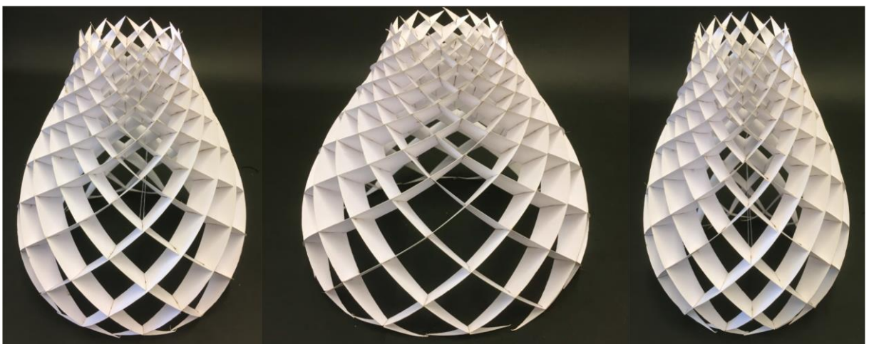
Figure 51 Paper model of the deformation of a rotational network with constant normal curvature (Schling, Kilian, et al., 2018).
