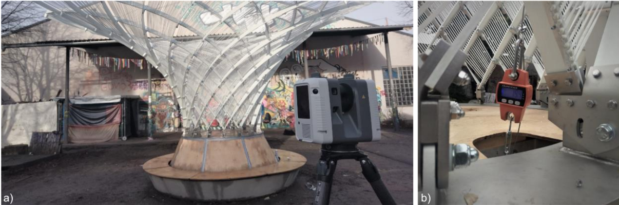
Figure 143 Measurements at the Kinetic Umbrella: a) Setup of lasers scan, b) Force meter interconnected at actuation cable
