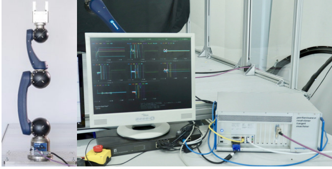
FIGURE 1. The testbed consists of a 6-DOF robot manipulator and a controller running on Simulink Real-Time.
