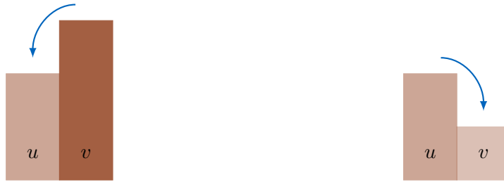
Figure 3.2.: The instance consists of two nodes u and v , where v is the higher of the two nodes. This means that water flows from v to u , which is illustrated on the left-hand side. If a basin with depth strictly larger than the absolute difference of the nodes' geodesic heights is built on v , the resulting geodesic height of v after building the basin is less than the geodesic height of u . Therefore, the water flows in the opposite direction after building the basin, which is illustrated on the right-hand side.
