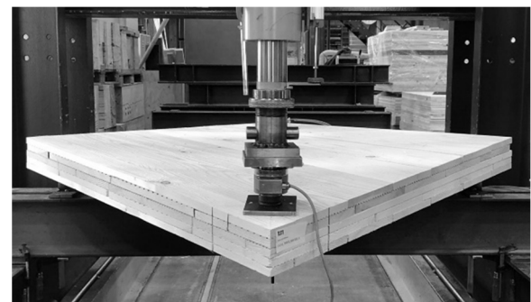
Figure 104: Biaxial bending tests to determine the torsional stiffness of CLT, DLT, and NLT specimens
