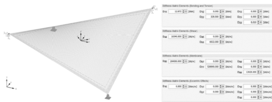
Figure 14: FEM shell model created with Dlubal RFEM [3]
