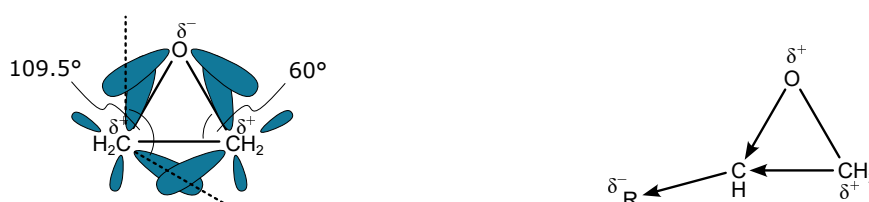
Figure 2.7: left: atomic orbital overlap and ring angle strain, [145] right: effect of a electron-withdrawing group. [142]
