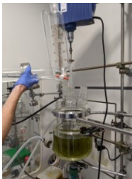
Figure A41: Glass reactor used for synthesizing epoxidized vegetable oils with formic acid and hydrogen peroxide.
