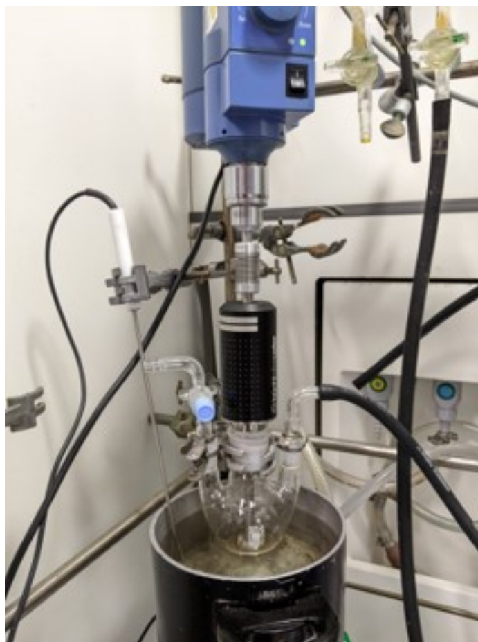
Figure A40: Reactor setup for polycondensation reactions. Three necked flask with vacuum-tight overhead stirrer and a vacuum receiver connector.
