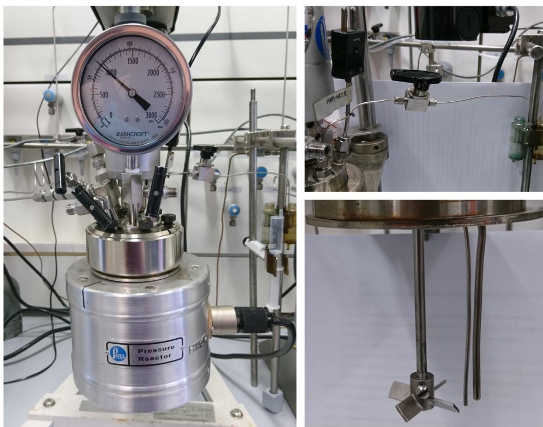
Figure 2: Experimental set-up of the autoclave. Left: fully assembled autoclave, including heater. Top right: pipe and 2-way valve used for sampling. Bottom right: stirring, thermocouple and sampling pipe attached to autoclave head.
