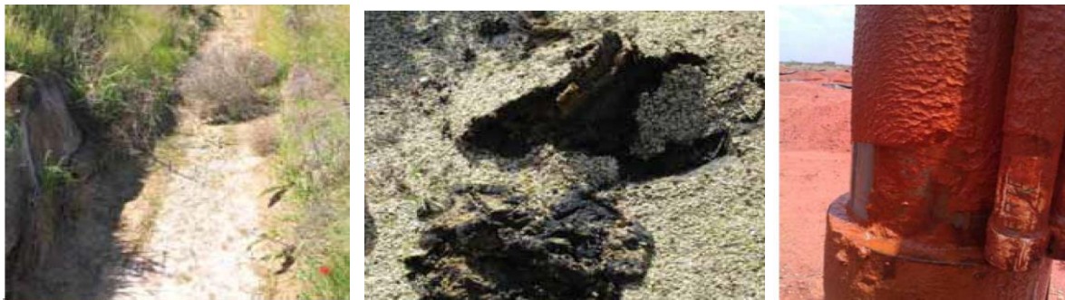
Figure 2: Types of clogging (physical, biological and chemical) at MAR sites, from Escalante (2013) and Willis-Jones and Brandes de Roos (2013).
