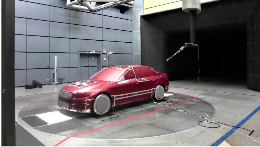
Figure 5: Vehicle in the Audi Aeroacoustic Wind Tunnel.
