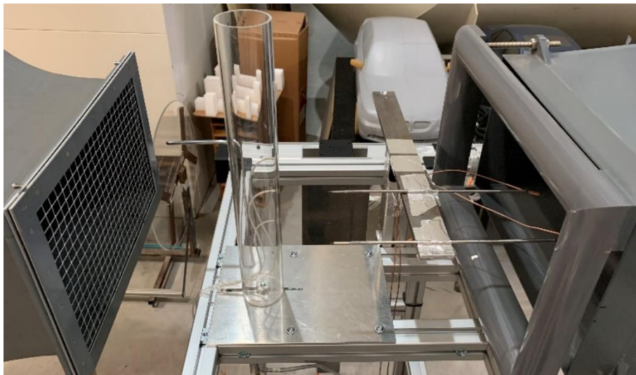
Figure 23: Top side view of cylinder in the model wind tunnel.
