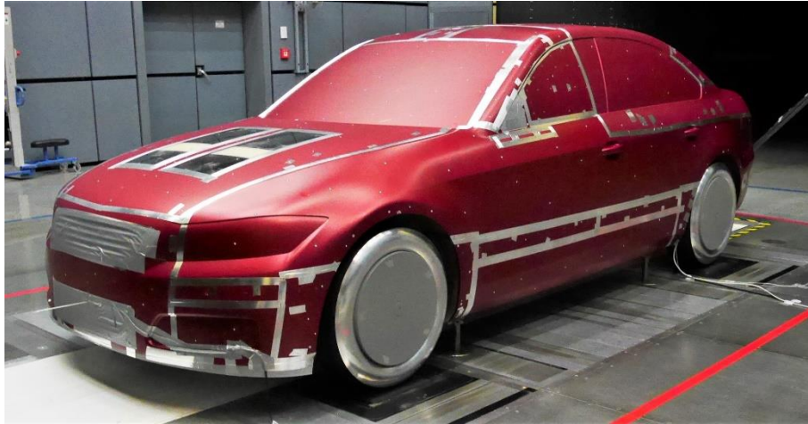
Figure 8: DrivAer with aluminium wheels and closed rims in the AAWT.
