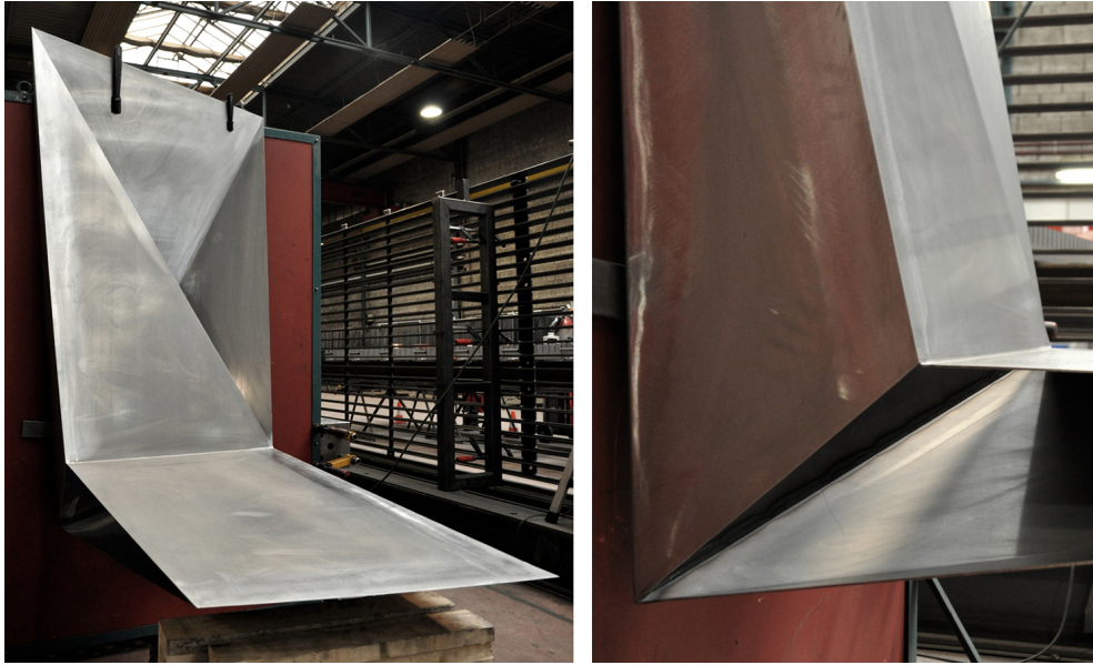
Figure 15.11: The foldDESK under construction. (Left) Overall view. (Right) Detail of the connection between the plates.
