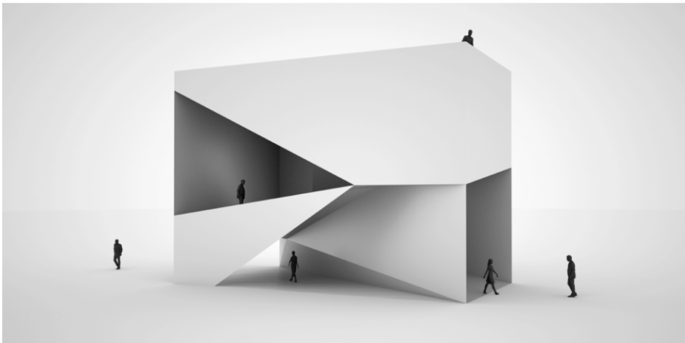
Figure 14.1: Series of folded plate prototypes at various scales designed using the proposed method for structural folding in architecture (Chapter 11).
