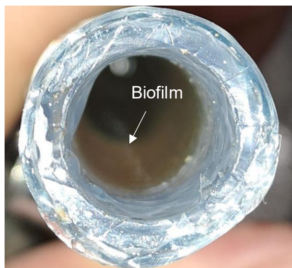
Figure 8-3: a) Biofilm first membrane element in series, experiment without UV pre-treatment; b) Feed pipe after the experiment with UV pre-treatment.
