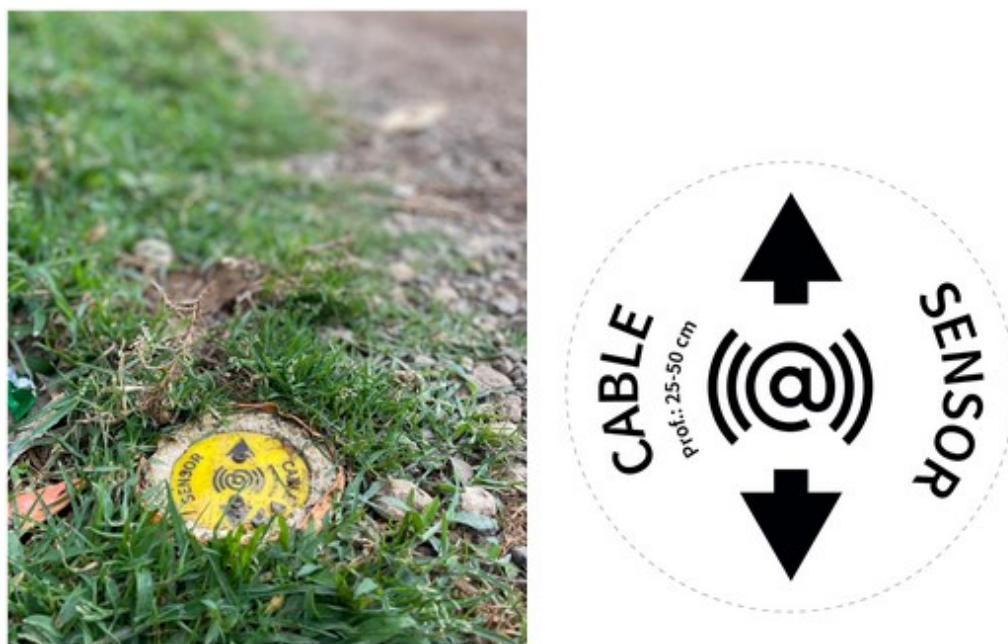
Figure 9. Point markers indicate the location of the horizontal CSM lines.
