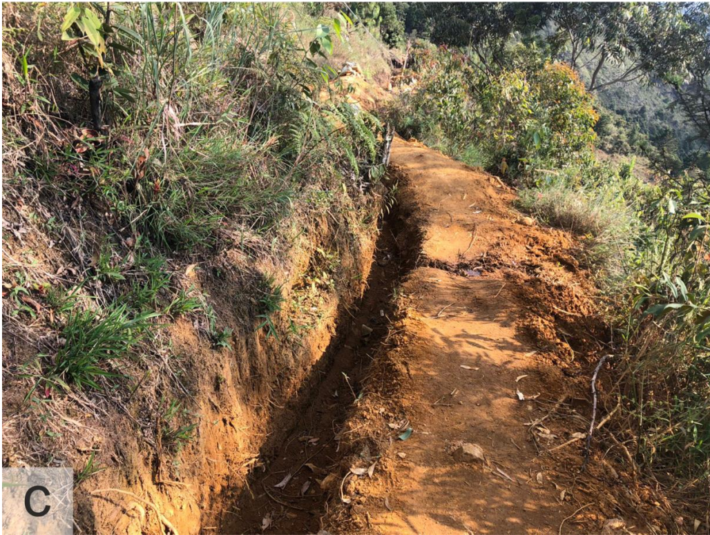
255 Figure 4: (a) Blocky material on the surface; (b) karstic holes under the excavated trench on 256 the upper part of the area; (c) trench in relatively undisturbed saprolite material with a lack of 257 large blocks. Pictures by (a) Josefina Ziegler, (b) Carolina Garcia-Londoño, (c) David Ceron.
