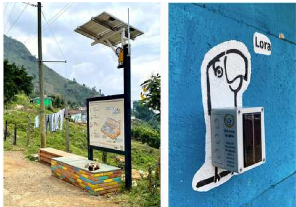
Figure 8. (Left): Gateway B functions as a small public space, with a large bench and an information sign. (Right): LoRa ® infrastructure node combined with a wall painting: “Lora the parrot” embodies the sensor.
