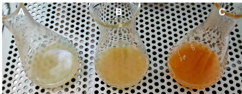
Figure 3. Visual difference between type I and II Fenton reactions (end of reaction). (A): Type II that failed to initialize boiling. (B): Type II which initialized boiling. (C): Type I.
