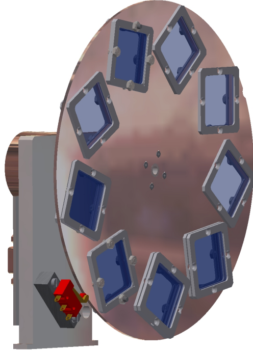
Figure 14: Original mechanical drawing of the target wheel. In the S444 experiment, the target wheel hosts 7 different targets and a large cut-out for background measurements.
