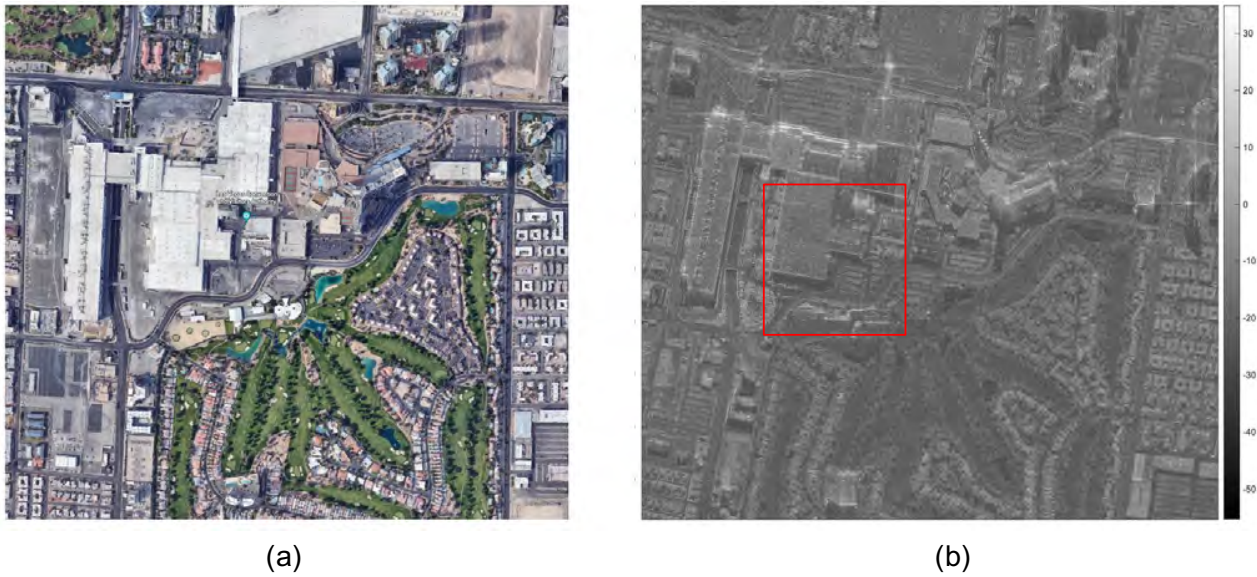
Fig. 10: Demonstration of the large test area. (a) Optical image from Google Earth, (b) SAR mean intensity map in dB. The red box in (b) indicates the area undergoing subsidence.
