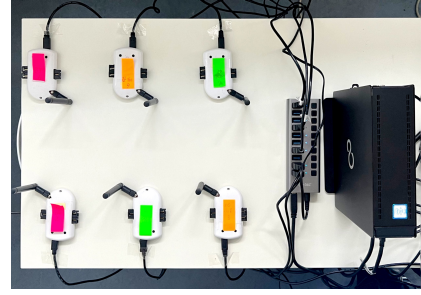
Fig. 3: The demonstration testbed. Six Zolertia ReMote sensors communicate over the shared wireless network. The control loops are closed over a mini PC.
