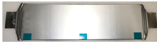
Figure 1. Cell under investigation. The pouch cell has large cell tabs on the sides, with which it can be electrically connected when testing modules. It can be seen that length \gg height \gg width .
