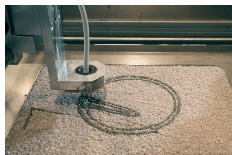
Figure 2. Selective paste intrusion (SPI) printer used for the investigations [36].
