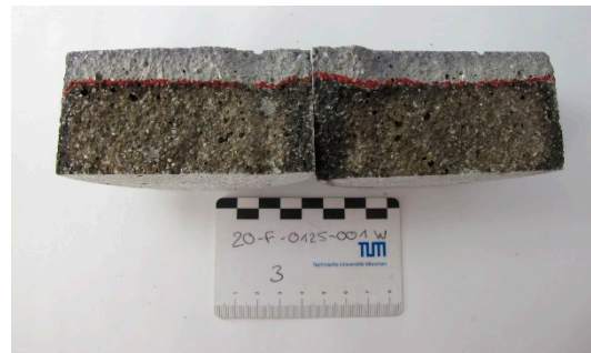
Figure 9. Cross-section of a 3D-printed D_{RCM} specimen (tested in 90^\circ ); light gray color on top: area with penetrated chloride; dark gray/brown color below: area without chloride.
