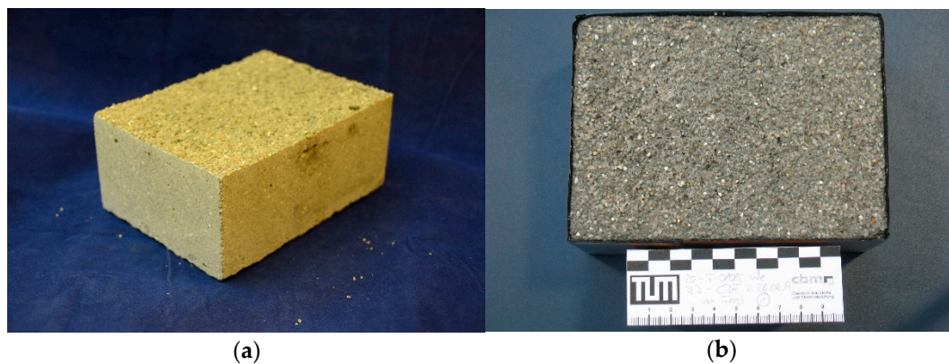
Figure 8. 3D printed ( 90^\circ ) specimen with (CDF) and without (CIF) deicing salt (a) with already sawn edges before sealing with Teflon tape with untreated test surface and (b) sealed with Teflon tape.
