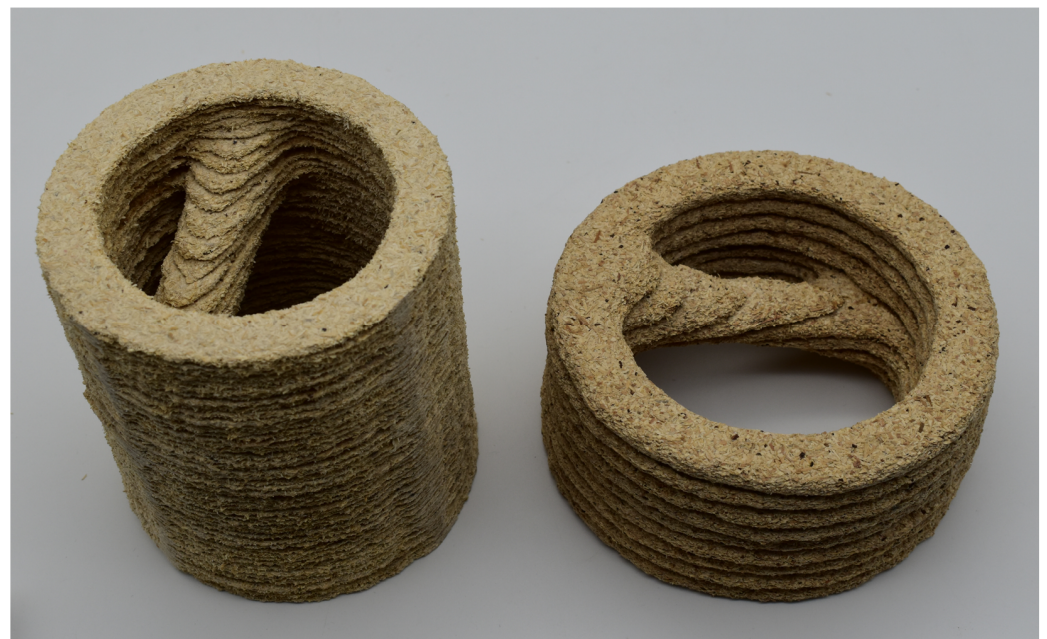
Figure 2. Demonstration objects for the ILF process with different panel thicknesses. While the panels were produced as described in the following sections, stacking and lamination were performed by hand with an epoxy resin as a binder.
