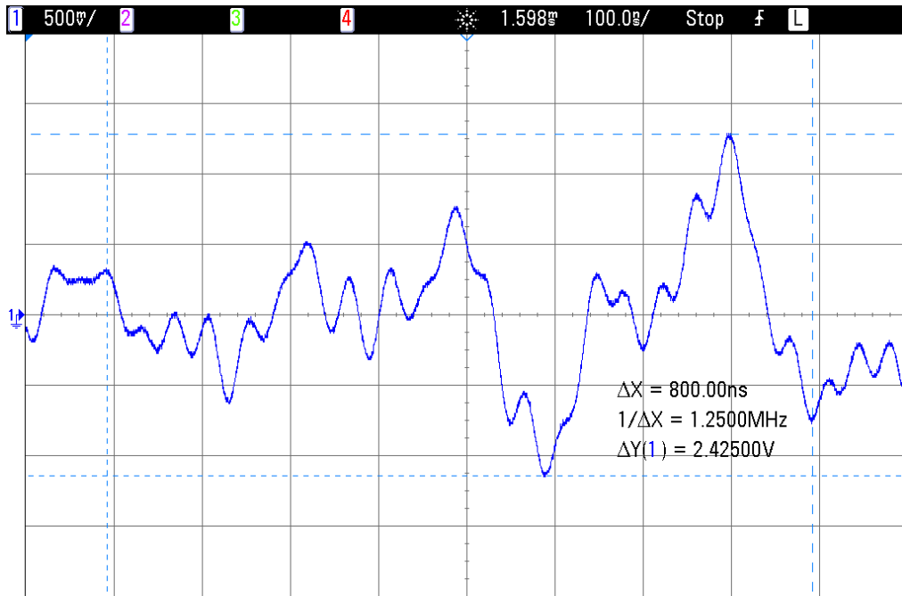
Figure 3.10: Zoom on a part of a HomePlug AV PPDU in time domain.
