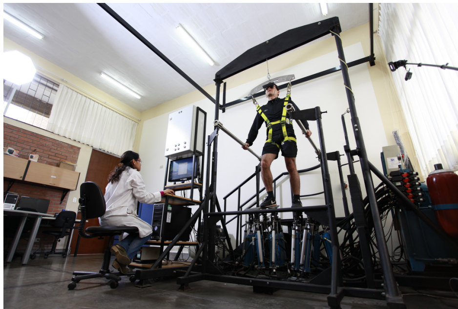
Figure 1. Gait simulator based on two Stewart–Gough platforms. During therapy, a user stands on both platforms, while a therapist supervises the system operation. Several safety measures have been implemented to protect the patient. A schematic describing the elements presented in this figure is provided in Figure 2.
