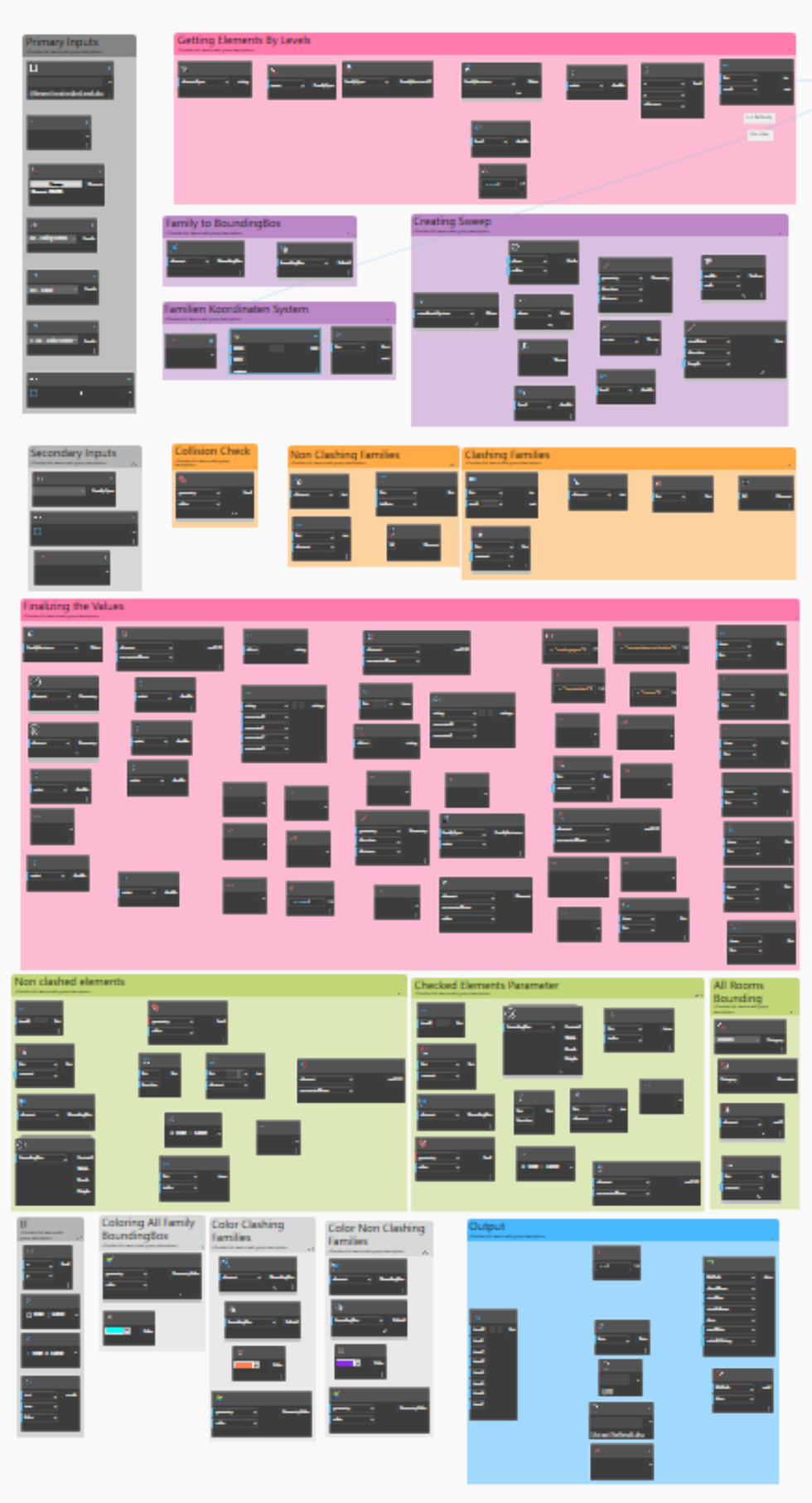
Figure 4. 6: The Dynamo script to check the position of the elements
