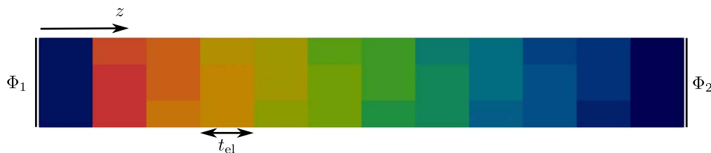
Figure 9. Regularly arranged solid electrolyte grains (colored domains). The grain boundaries occur between the solid electrolyte grains. The difference in electric potential is \Delta\Phi_{el} = \Phi_2 - \Phi_1 .
