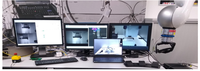
Fig. 7. Workplace for the human teleoperator. A LWR arm in mirrored joint configuration is used as haptic input device (top right section of the image). Different camera views (right screen: front view, middle screen: top view and visualization, laptop: side view) are available for the operator. The left screen displays the vision detection algorithm and is hidden during the user study.
