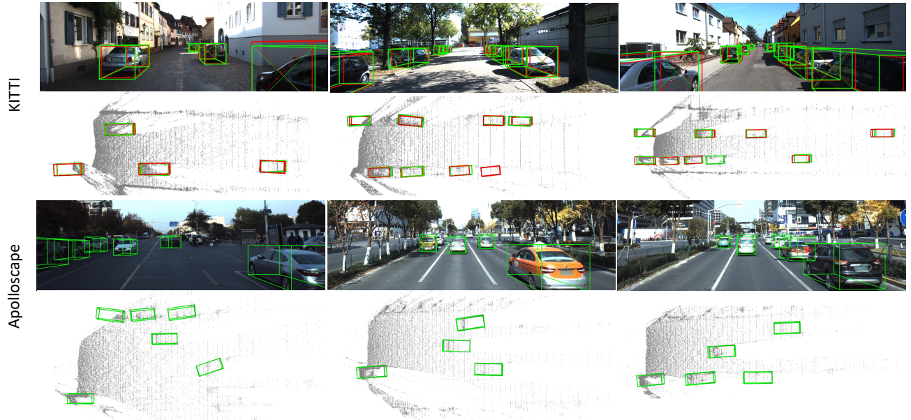
Fig. 5: Qualitative results of ER3D on the two datasets. The top two rows illustrate the prediction and the ground truth of the KITTI dataset and the bottom two rows show the 3D detection results on the ApolloScape dataset. The predictions of ER3D are illustrated as green and the ground truth 3D labels are illustrated as red . The depth of SGM is utilized to generate the point cloud in the first and the third row.
