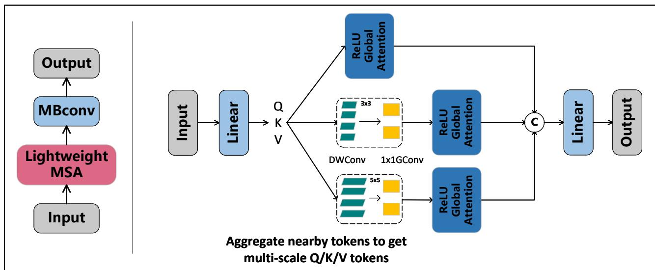
**Figure 5.** EfficientViT module structure.
