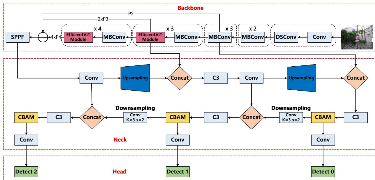
**Figure 2.** YOLOv5 -EfficientViT (Ours) object detection model structure.
