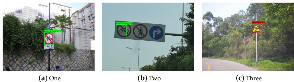
**Figure 14.** YOLOv4-tiny object detection model output results.
