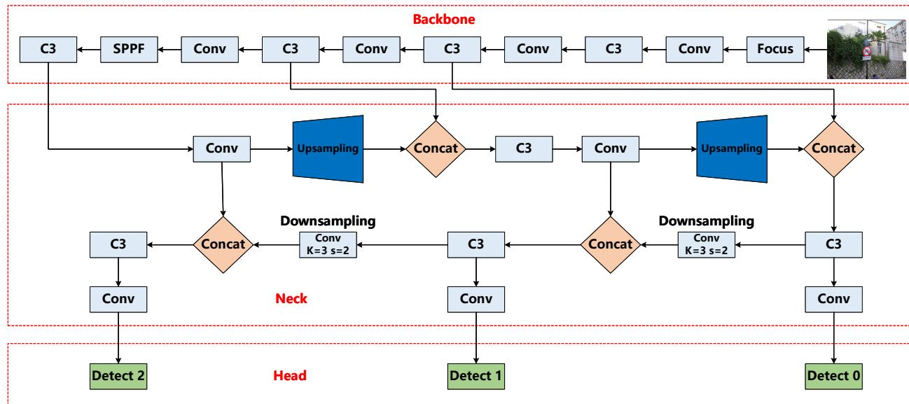
**Figure 1.** YOLOv5(s) object detection model structure.
