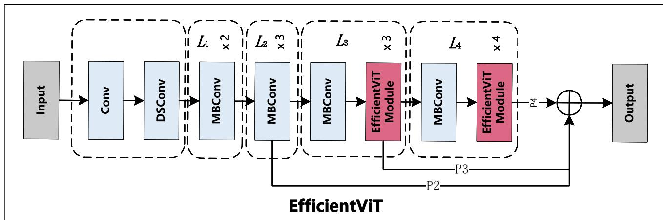
**Figure 3.** EfficientViT general structure.
