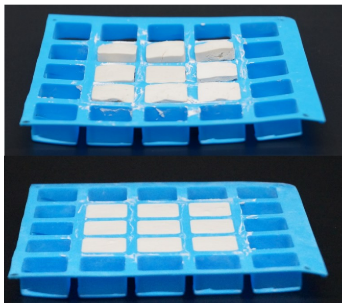
Figure 3 Silicon mould after microwave treatment with P1 (top) and P2 (bottom).
