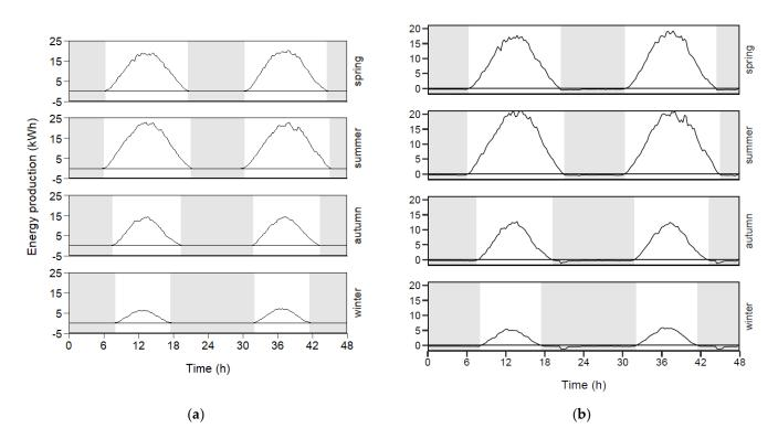
**Figure 2.** Energy production of the PV plant in 15 min resolution for a 48.00 h period (**a**); energy balance of the milk production system and the PV plant in a 48.00 h period (**b**). Periods with negative energy balance are indicated with grey areas.
