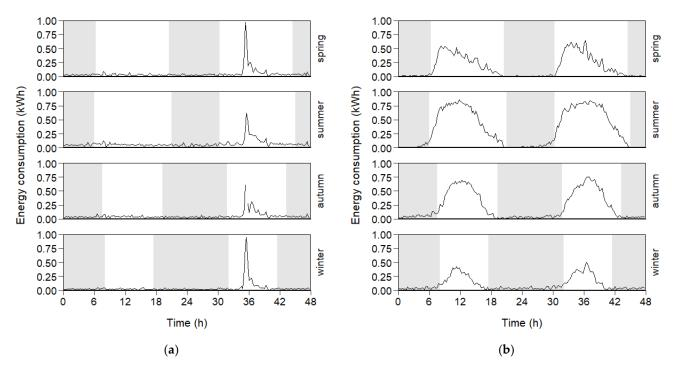
**Figure 7.** Mean energy consumption of the milk cooling tank (**a**) and cooling unit (**b**) during 48.00 h period with a resolution of 15 min; periods with negative energy balance are indicated with grey areas.
