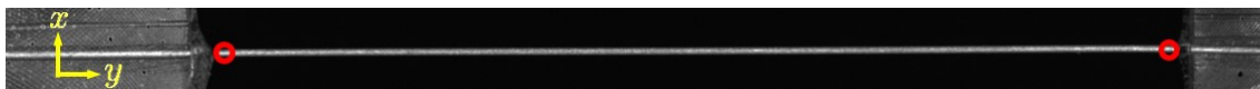
Figure 6.5: Image of a tungsten wire with a diameter of 150\ \mu\text{m} during a mechanical test. The regions of interest that were tracked are indicated by red circles.
