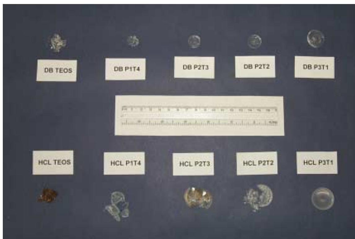
Figure 5.3 Monoliths obtained by sol-gel process
