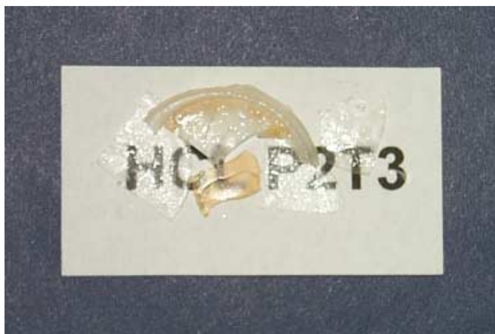
Figure 5.7 Monolith HCLP2T3, full phase separation between silica (yellow) and polymethylmethacrylate.
