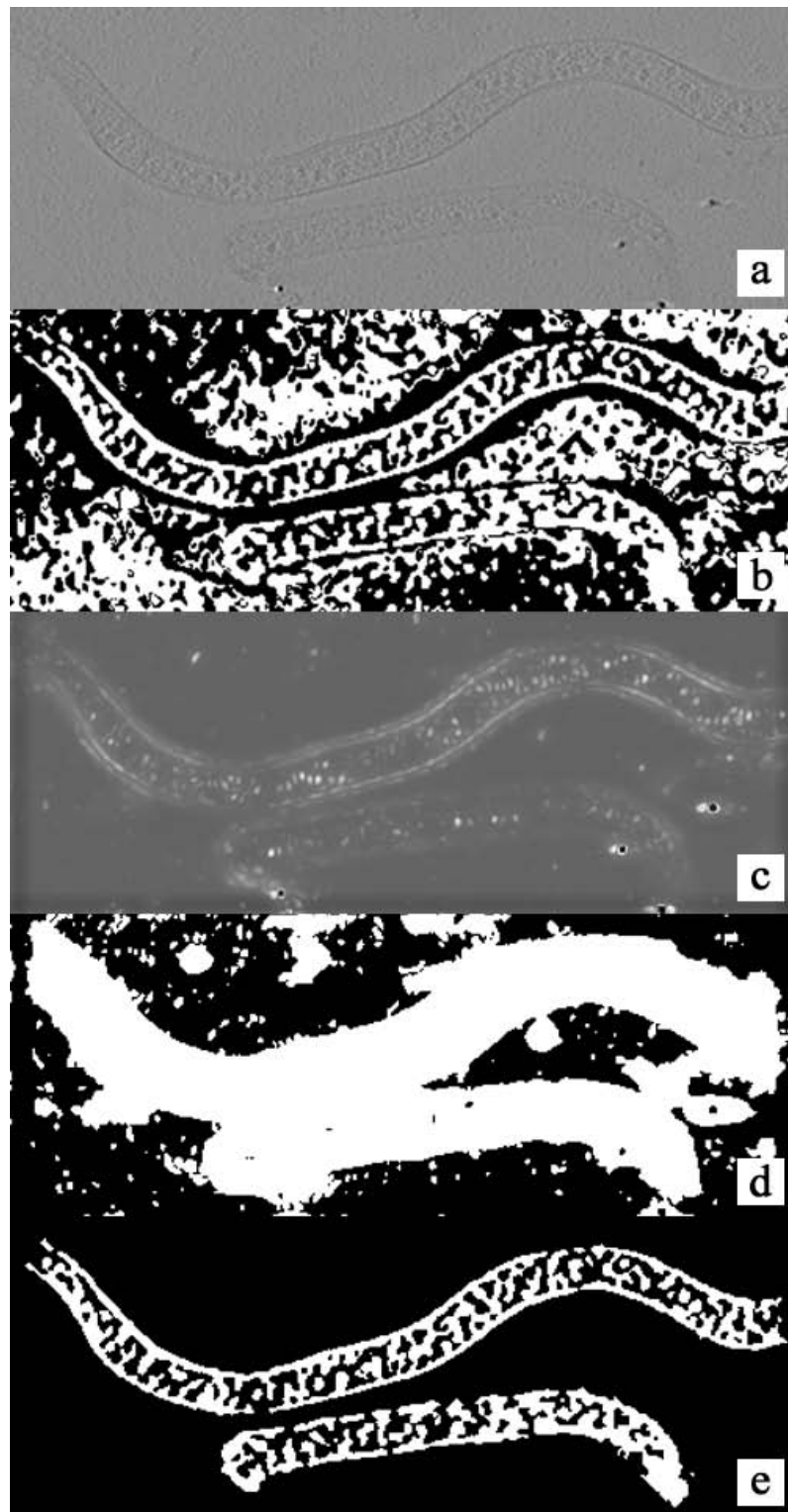
Figure 4.13: Segmentation of S. melliferum a) 2-D XY-slice of the original tomogram after denoising with N.A.D., b) segmentation by simple thresholding of the gray-values, c) calculation of the scaling indices for r = 15 , d) thresholding of the scaling indices, and e) final segmentation mask.
