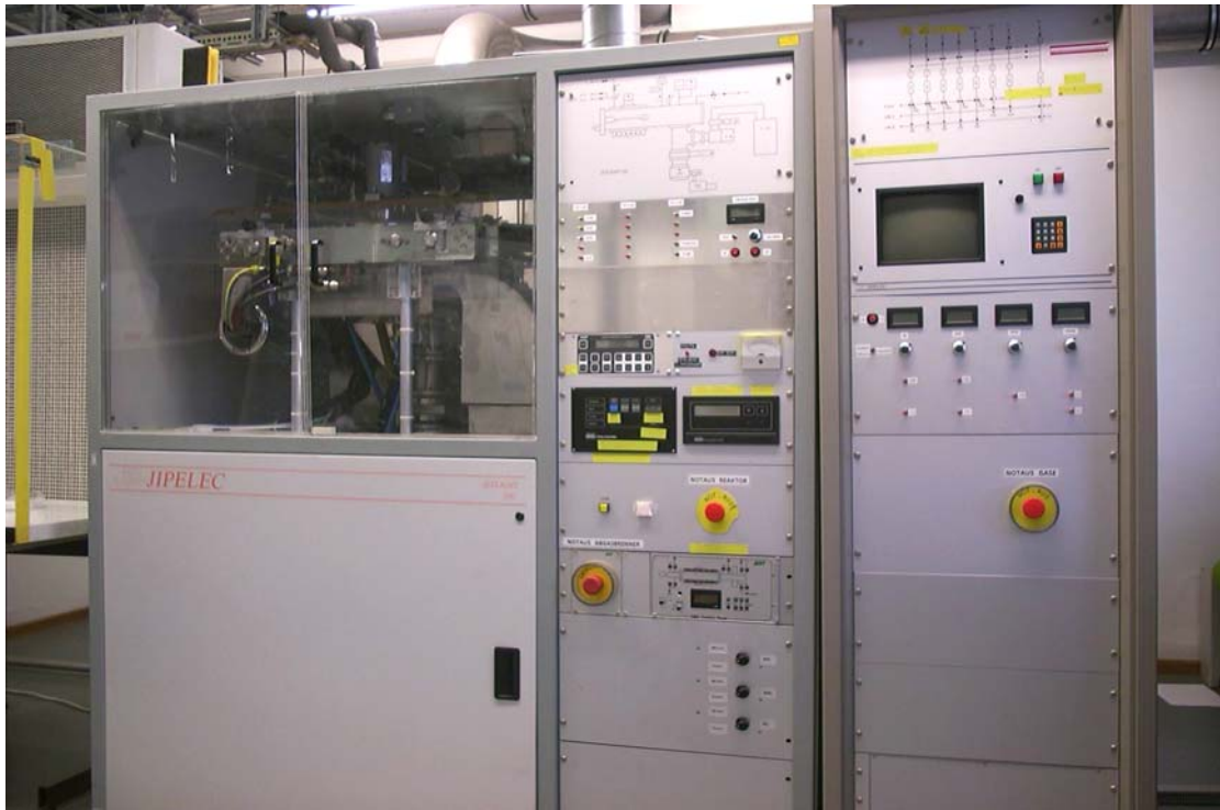
Fig. 4-22 Picture of the RTCVD system (JETLIGHT 200)
