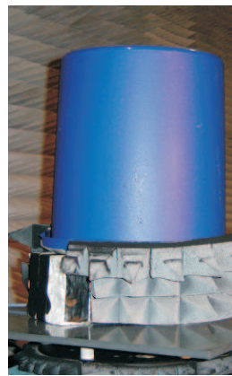
(ii) Conformal dipole antenna and cylindrical reflector embedded into cylindrical radome.
