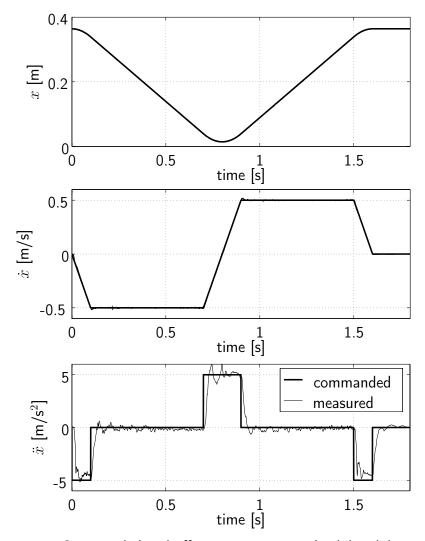
Figure 5.9: Commanded end-effector trajectory at backdrivability experiment
