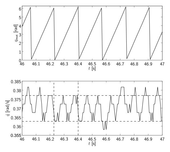
Figure 4.22: Joint velocity progression measured for a constant actuation torque of  $2.8\,\mathrm{N\,m}$  (joint 3 of VISHARD3). Velocity oscillation points to position dependency of friction.
