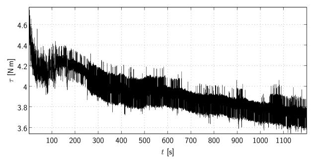
**Figure 4.13:** Variation of friction with time (joint 3 of VISHARD3,  $\dot{q} = \pi \, \text{rad/s}$ )
