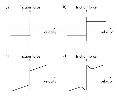
Figure 4.1: Static friction models: a) Coulomb friction; b) Coulomb plus static friction; c) Coulomb plus static plus viscous friction; d) Coulomb plus viscous friction plus Stribeck effect.
