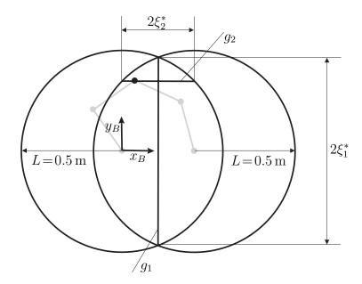
Figure 3.11: Coding of the joint 3 position to obtain a rectangular search space
