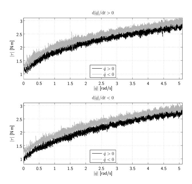
Figure 4.16: Symmetry of the Stribeck curve ( $32 \,^{\circ}\text{C}$ , joint 6 of the 7 DOF telemanipulator presented in [SB04])
