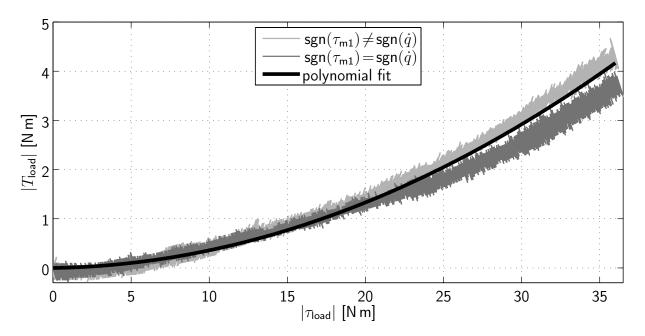
Figure 4.21: Load dependent friction torque of the VISHARD3 joints
