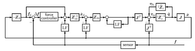
Figure 4.12: Rearranged diagram of impedance control with disturbance observer
