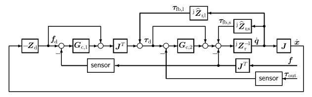
Figure 4.10: Impedance control with endpoint force and joint torque feedback
