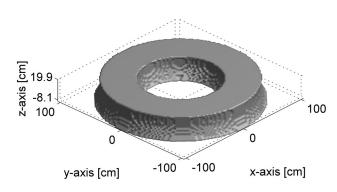
Figure 2.1: VISHARD6 prototype (left) and its singularity free translational workspace for an orientation workspace of  $360^{\circ}$ ,  $90^{\circ}$ , and  $360^{\circ}$  for the angle of roll, pitch, and yaw, respectively (right)
