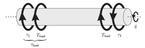
Figure 4.20: Torque balance: the load dependent friction  $T_{load}$  opposes the motion  $\dot{q}$ .
