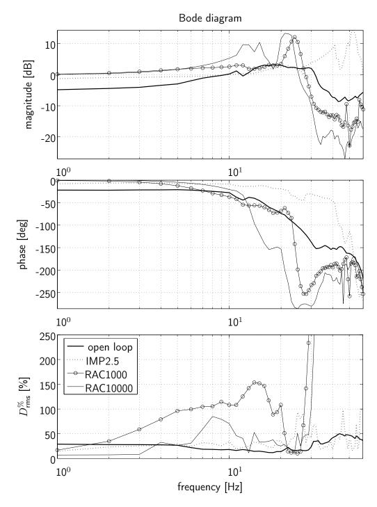
**Figure 5.13:** Force frequency response of impedance and admittance control laws: magnitude, phase, and signal distortion
