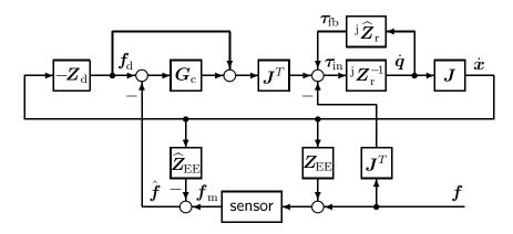
Figure 3.4: Impedance control with force feedback and model-based compensation
