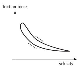
**Figure 4.4:** Frictional lag: Friction-velocity relation for unidirectional sinusoidal velocity input within the partial fluid lubrication regime
