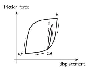
**Figure 4.3:** Pre-sliding hysteresis: Typical static friction for a displacement trajectory within the elastic pre-sliding displacement regime; the motion starts from point a, follows b-c-d-e and arrives at point f
