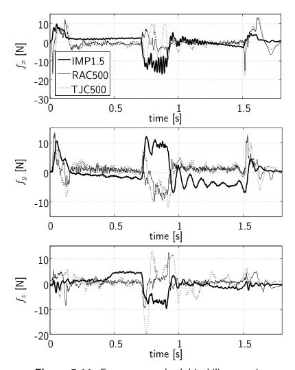
Figure 5.11: Force error at backdrivability experiment
