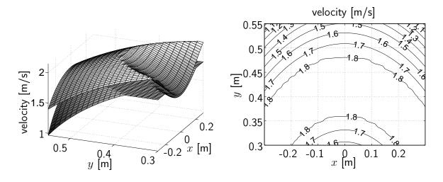
**Figure 5.2:** Velocity capability of VISHARD3; left: result for end-effector height  $z=\pm 0.20\,\mathrm{m}$  (worst case) and  $z=0\,\mathrm{m}$  (best case); right: contour plot for worst case result
