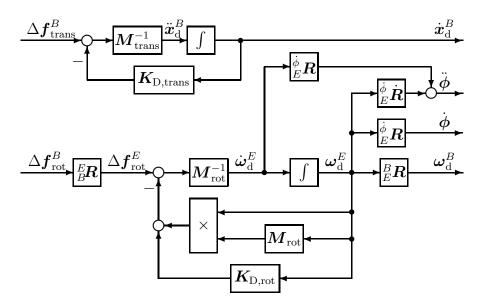
**Figure 3.8:** Implementation of virtual admittance  $oldsymbol{Z}_{d2}^{-1}$
