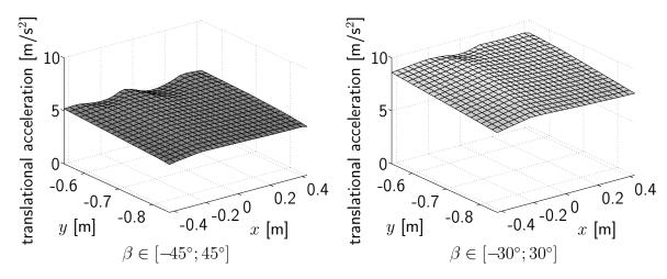
**Figure 5.7:** Translational acceleration capability of VISHARD6 with  $\alpha, \gamma \in [-180^{\circ}; 180^{\circ}]$
