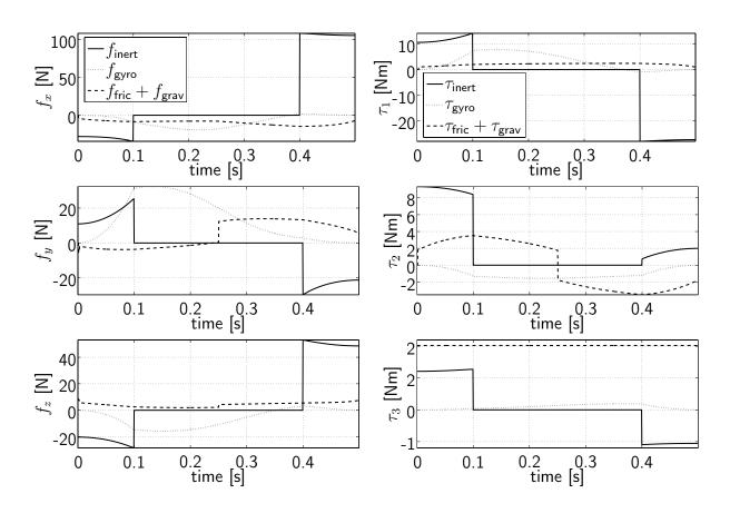
**Figure B.2:** Force/torque components due to inertial, gyroscopic, frictional, and gravitational effects
