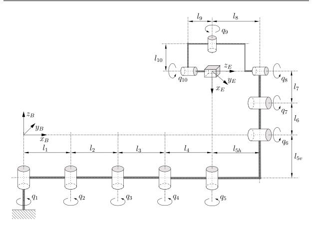
Figure 2.7: Kinematical model of VISHARD10
