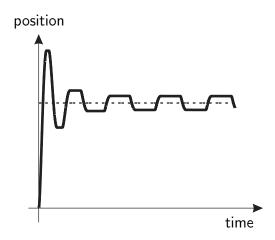
**Figure 4.7:** Hunting oscillations under PID position control; dashed line: desired position; solid line: actual position
