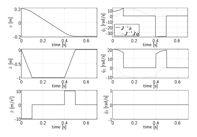
**Figure B.1:** Commanded end-effector trajectory and corresponding accelerations in the joint space
