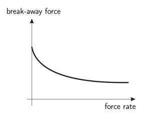
Figure 4.5: Dependency of the break-away force on the rate of force application
