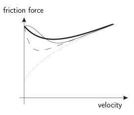
Figure 4.2: Effect of  $\delta$ ,  $v_{\rm s}$ , and  $f_{\rm s}$  on the shape of the Stribeck curve: the thick line is the reference Stribeck curve; thin: increased  $\delta$ ; dashed: decreased  $v_{\rm s}$ ; dotted: decreased  $f_{\rm s}$  ( $f_{\rm s} < f_{\rm c}$ )
