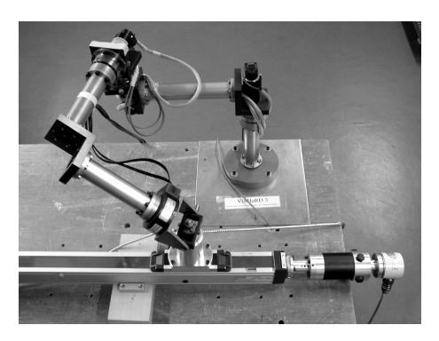
Figure 4.23: VISHARD3 coupled to a linear guide
