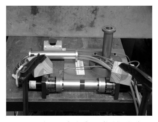
Figure 4.19: Hardware setup for identification of load dependent friction
