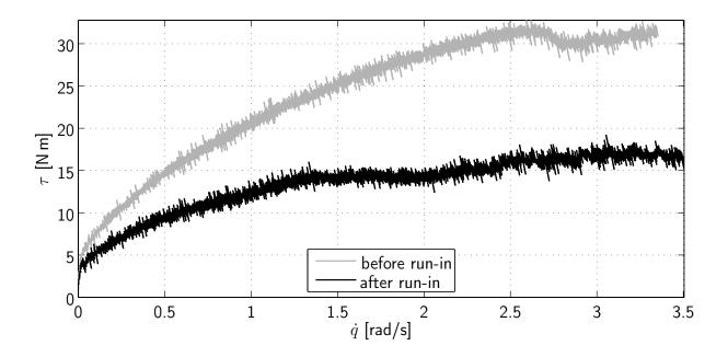
Figure 4.17: Change of frictional behavior during the run-in period (joint 1 of VISHARD10)
