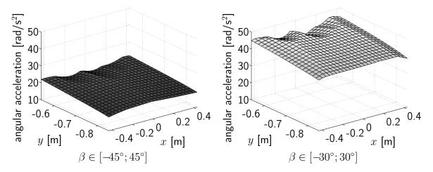
**Figure 5.8:** Angular acceleration capability of VISHARD6 with  $\alpha, \gamma \in [-180^{\circ}; 180^{\circ}]$
