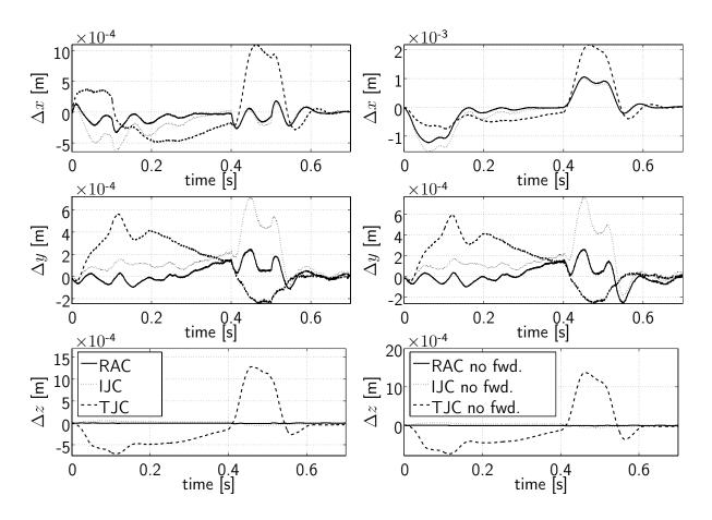
**Figure B.3:** Position tracking errors; left: control with acceleration feedforward; right: control without acceleration feedforward
