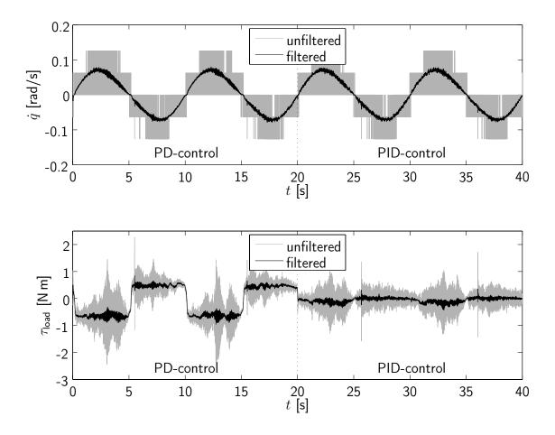
Figure 4.24: Stiction compensation: Friction reduction at very low velocities through addition of integral action to the PD control-law (joint 2 of VISHARD3)
