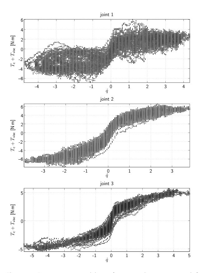
Figure 4.25: Friction torques estimated during a free space simulation in a time period of forty seconds
