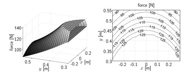
Figure 5.1: Peak force capability of VISHARD3; left: result for end-effector height  $z=0\,\mathrm{m}$  (worst case) and  $z=\pm0.20\,\mathrm{m}$  (best case); right: contour plot for worst case result
