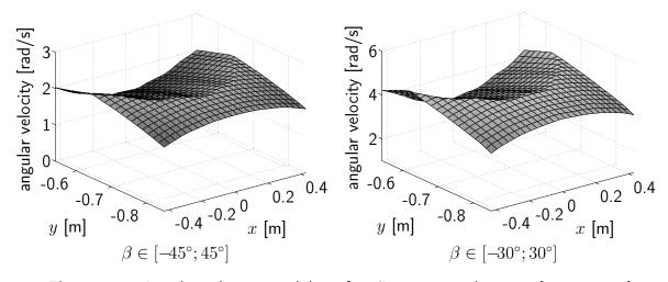
**Figure 5.6:** Angular velocity capability of VISHARD6 with  $\alpha, \gamma \in [-180^{\circ}; 180^{\circ}]$
