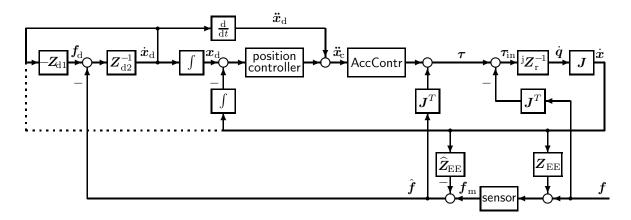
Figure 3.5: Admittance control; dashed line indicates position-based impedance control
