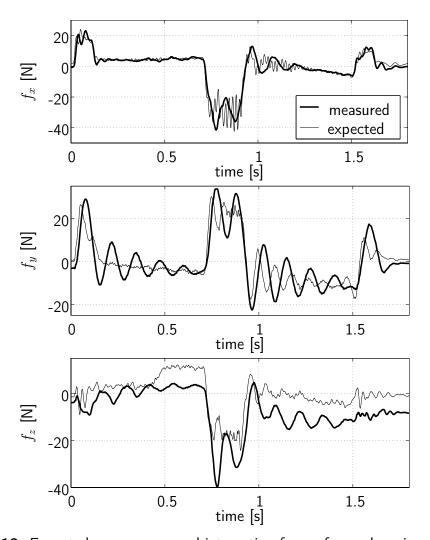
Figure 5.12: Expected versus measured interaction force of open loop impedance control
