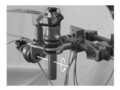
Figure 3.9: Critical end-effector motion: rotation around the axis of joint 9 drives the wrist towards a singular configuration producing high accelerations of joint 5
