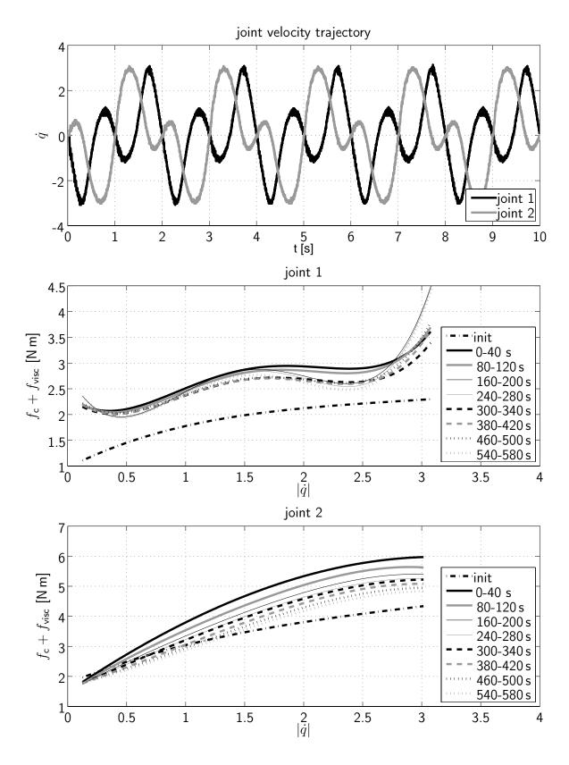
Figure 4.27: Estimation of the VISHARD3 Stribeck curve during motions induced by a linear guide
