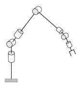
Figure 2.6: Typical 7 DOF anthropomorphic robot arm
