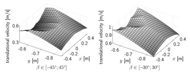
**Figure 5.5:** Translational velocity capability of VISHARD6 with  $\alpha, \gamma \in [-180^{\circ}; 180^{\circ}]$
