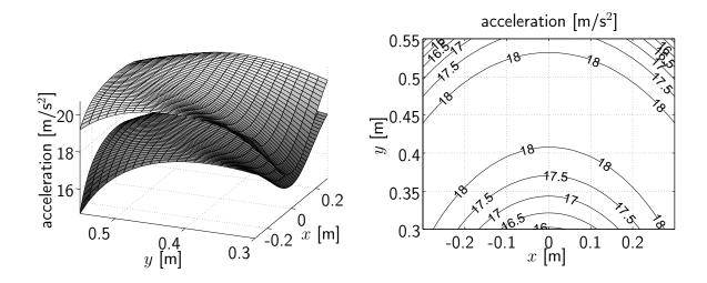
Figure 5.3: Acceleration capability of VISHARD3: ; left: result for end-effector height  $z=\pm 0.20\,\mathrm{m}$  (worst case) and  $z=0\,\mathrm{m}$  (best case); right: contour plot for worst case result
