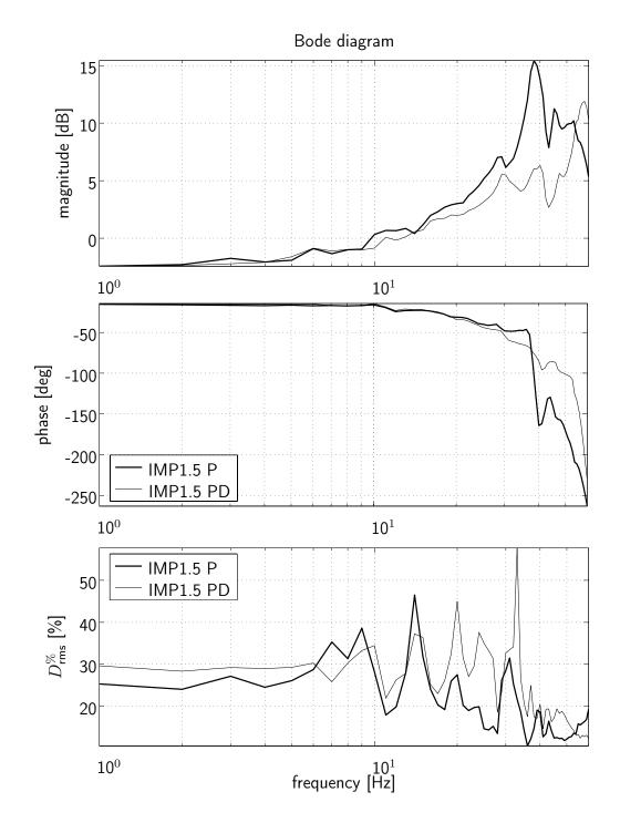
Figure 5.14: Force frequency response of impedance control with and without derivative action
