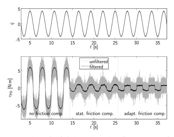
Figure 4.28: Reduction of the feedback control action due to friction compensation (joint 2 of the  ${
