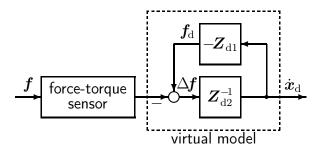
Figure 3.7: Virtual admittance implemented as coupling between impedance and admittance
