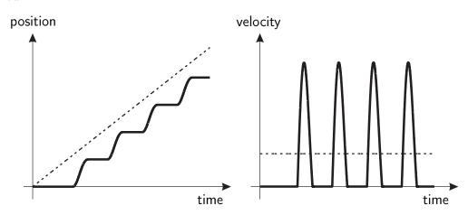
**Figure 4.6:** Stick-slip motion at low constant velocity tracking under PD position control; dashed line: desired motion; solid line: actual motion
