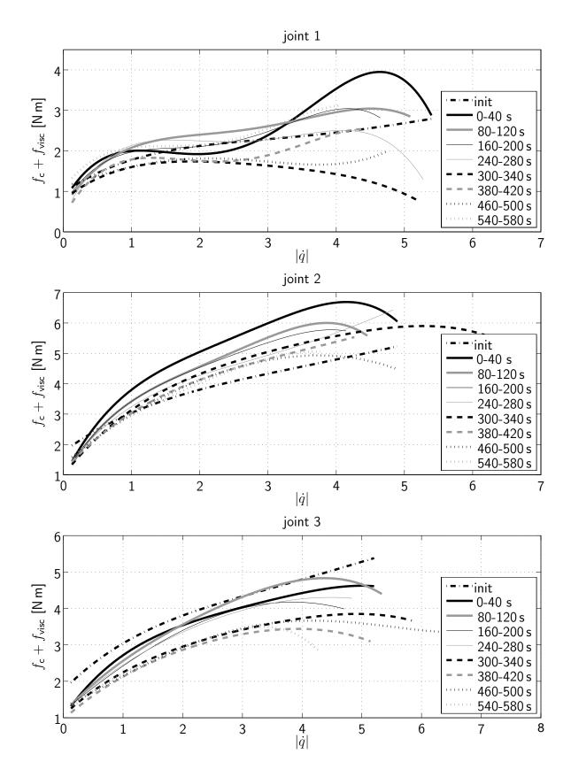
Figure 4.26: Estimation of the VISHARD3 Stribeck curve during motions induced by a human operator
