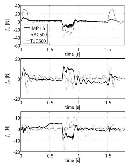
Figure 5.10: Interaction force at backdrivability experiment
