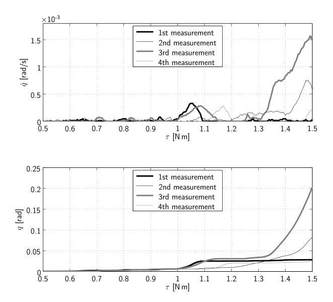
Figure 4.18: Results of break-away force identification experiments (joint 1 of VISHARD3).
