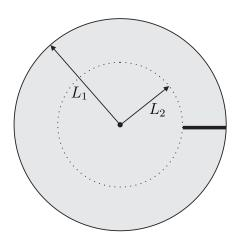
Figure 3.10: Exclusion of workspace area (thick line) to satisfy Wampler's necessary conditions for invertibility;  $L_1 = 0.85 \,\mathrm{m}$ ,  $L_2 = 0.5 \,\mathrm{m}$
