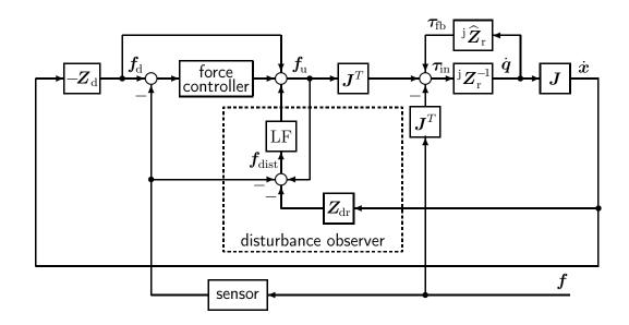
Figure 4.11: Impedance control with disturbance observer
