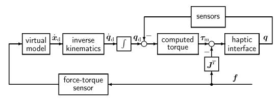
Figure 3.6: Admittance control scheme of VISHARD10
