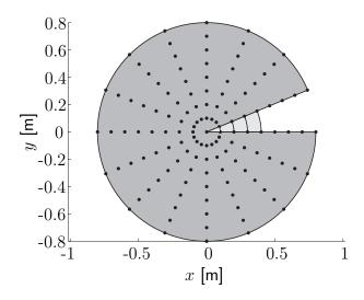
Figure 3.12: Inverted workspace; the dots indicate the mesh of end-effector positions considered in the optimization routine
