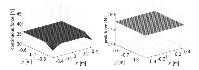
Figure 5.4: Continuous and peak force capability of VISHARD6 with  $\alpha, \gamma \in [-180^\circ; 180^\circ]$  and  $\beta \in [-45^\circ; 45^\circ]$
