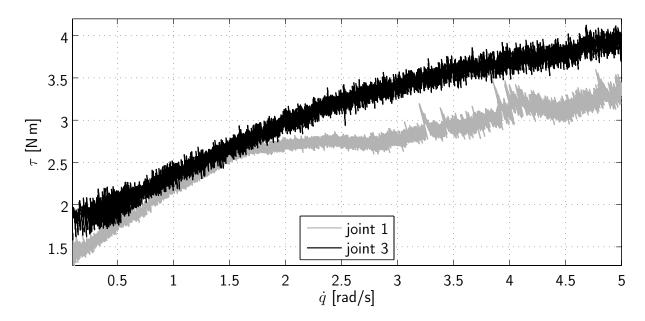
Figure 4.14: Stribeck curve of joint 1 and 3 of the VISHARD3 device
