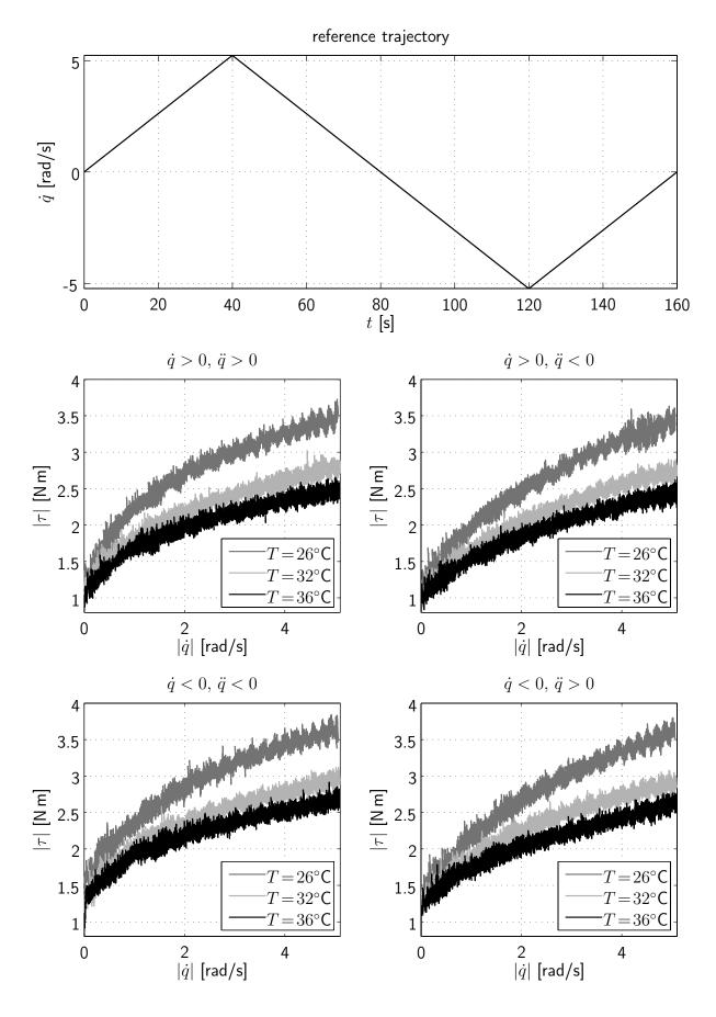
Figure 4.15: Temperature dependency of the Stribeck curve (joint 6 of the 7 DOF telemanipulator presented in [SB04])
