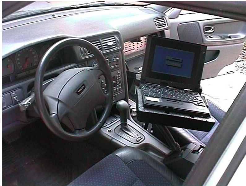
Figure 8.1: View of the Volvo Demonstrator Car showing the notebook connected to the ECU
