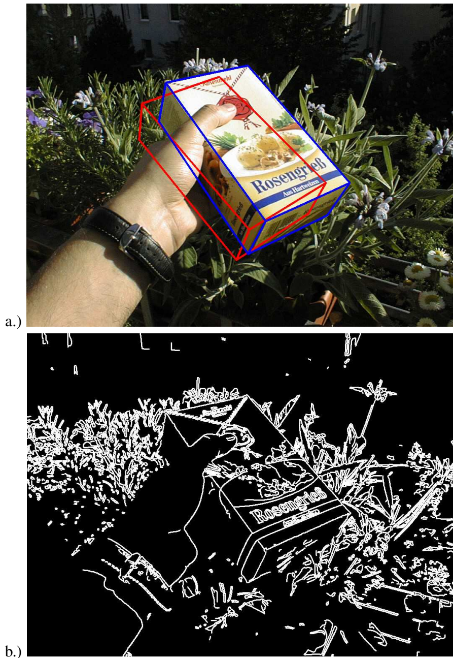
Figure 5.12: Partially occluded box in front of an inhomogeneous background: a.) Due to the directed illumination, the contrast between the background and the box heavily varies. Nevertheless, the CCD algorithm accurately fits a wire frame model to the image data (red = initialization, blue = estimate). b.) Here again a gradient-based edge detector (Steger, 2000) yields multiple false positives and false negative errors.
