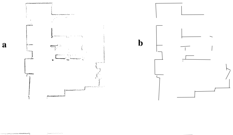
Figure 5.4: Generating 2D line segments maps from laser scan data, a - 5042 scan points from 30 scans, b - after line merging, 38 line segments
