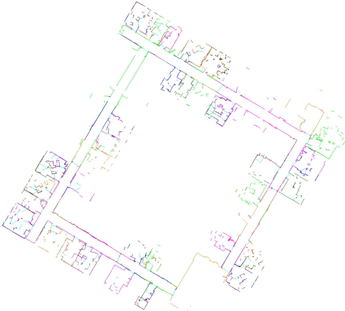
Figure 6.10: Department floor of Informatik IX, TU Munich (Orleanstr.). The data set comprises 2638 scans. The robot traveled a total of about 817 meter.
